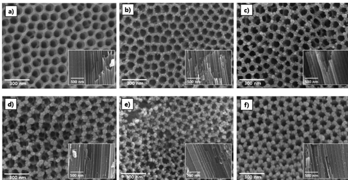
Fig. 7 FE-SEM images (cross sectional view in inset images) of (a) r-TiO<sub>2</sub> and RuO<sub>2</sub> coated electrodes after immersion in 5 mM aqueous ruthenium precursor for (b) 1, (c) 3, (d) 6, (e) 12, and (f) 24 h. Note that FE-SEM images of r-TiO<sub>2</sub> and RuO<sub>2</sub>@r-TiO<sub>2</sub> (24 h) were from the result of Fig. 2 in order to compare the morphologies of each electrode.
