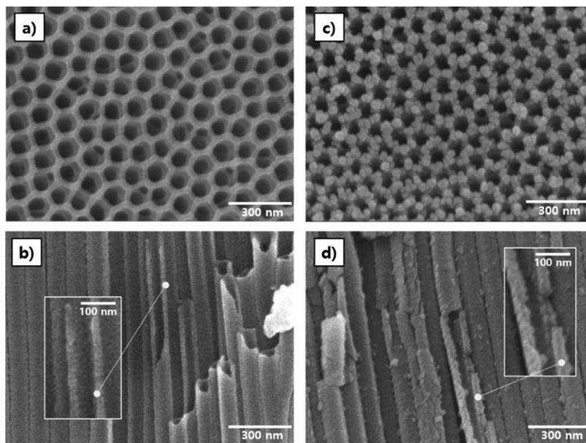
Fig. 2 Morphologies of (a) top- (b) cross sectional view of r-TiO<sub>2</sub> and (c) top- (d) cross sectional view of RuO<sub>2</sub>@r-TiO<sub>2</sub> with a field emission scanning electron microscope (FE-SEM).
