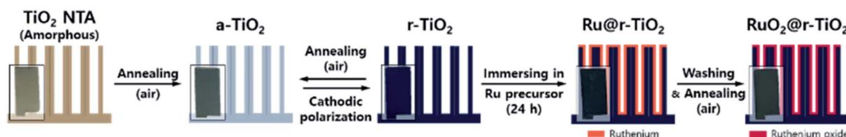
Fig. 1 Scheme of thin RuO<sub>2</sub> layer coating process on reduced TiO<sub>2</sub> nanotube array *via* electrochemical self-doping.
