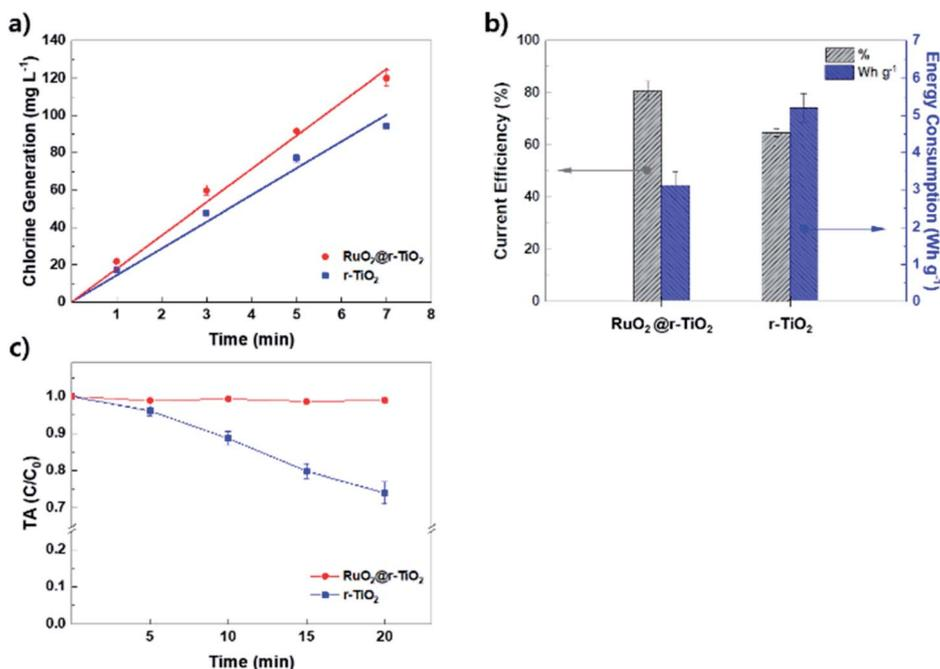
Fig. 6 (a) Evolution of chlorine (16.7 mA cm<sup>-2</sup>, 0.1 M NaCl) and (b) the current efficiency and energy consumption in 3 min, and (c) terephthalic acid (TA) degradation for hydroxyl radical measurement (0.1 mM TA, 16.7 mA cm<sup>-2</sup>) of RuO<sub>2</sub>@r-TiO<sub>2</sub> and r-TiO<sub>2</sub>.
