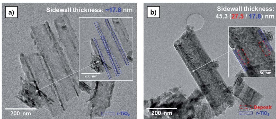
Fig. 3 Nanotube structure characterization of (a) r-TiO<sub>2</sub> and (b) RuO<sub>2</sub>@r-TiO<sub>2</sub> using field emission transmission electron microscope (FE-TEM).
