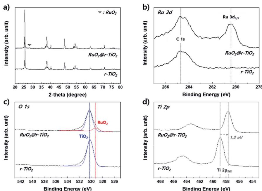
Fig. 4 (a) XRD patterns and XPS spectra (b) Ru 3d, (c) O 1s, and (d) Ti 2p of r-TiO<sub>2</sub> and RuO<sub>2</sub>@r-TiO<sub>2</sub>.
