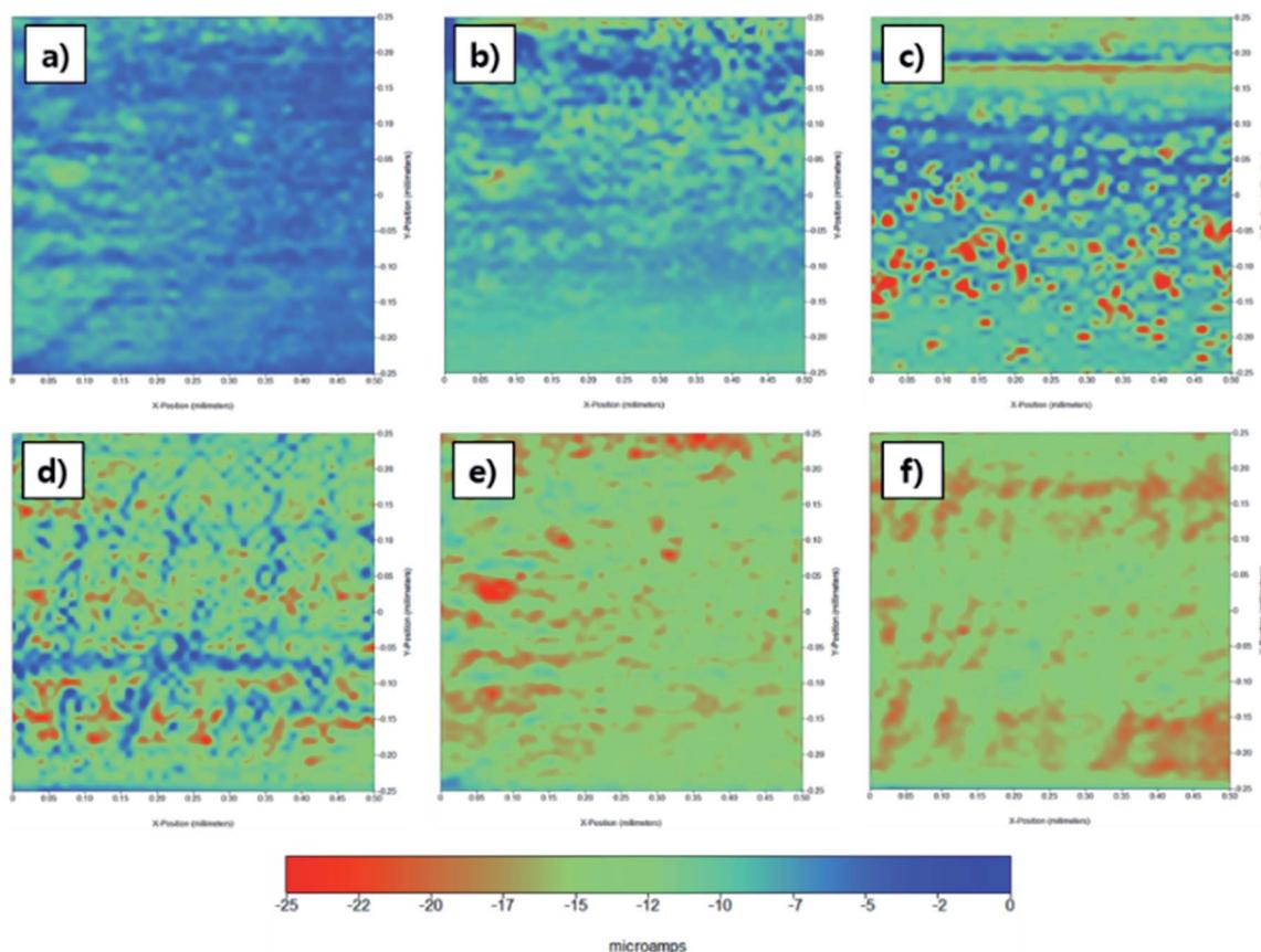
Fig. 9 Area scan of scanning electrochemical microscopy (SECM) in 0.1 M NaCl, 16.7 mA cm<sup>-2</sup>; (a) r-TiO<sub>2</sub>, RuO<sub>2</sub> coated electrodes after immersing in 5 mM aqueous ruthenium precursor for (b) 1, (c) 3, (d) 6, (e) 12, and (f) 24 h.
