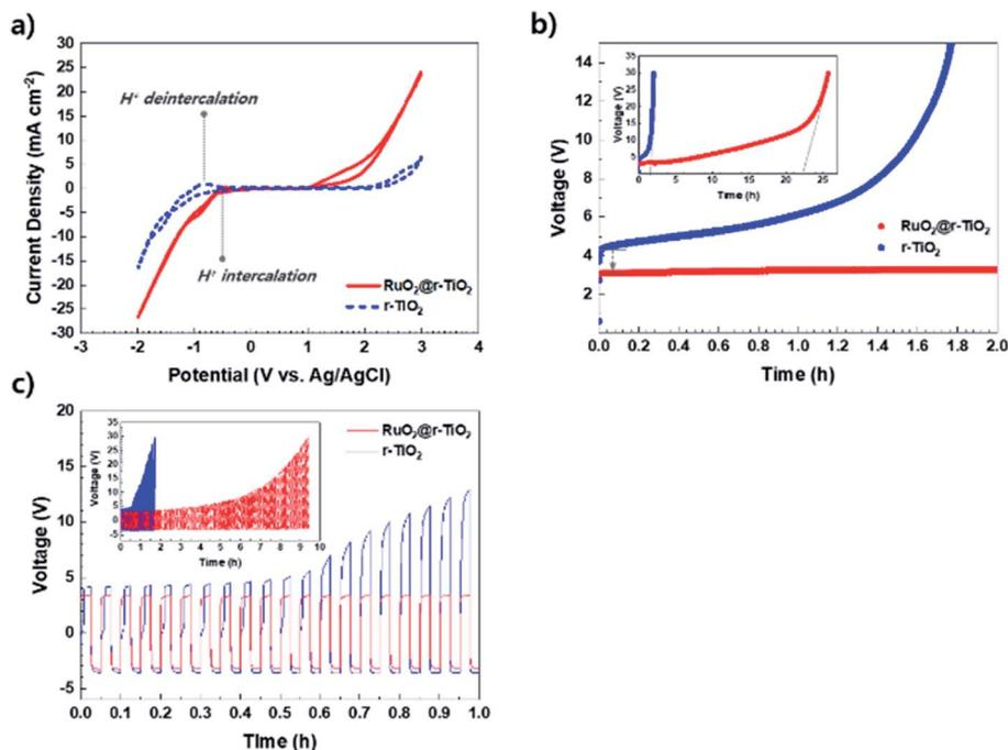
Fig. 5 (a) Cyclic voltammograms (CV) (scan rate: 5 mV s<sup>-1</sup>), the stability test with (b) applied constant current density (16.7 mA cm<sup>-2</sup>), and (c) polarity reversal operation ( $\pm 16.7$  mA cm<sup>-2</sup>, switching time 90 s) of r-TiO<sub>2</sub> and RuO<sub>2</sub>@r-TiO<sub>2</sub> in 0.1 M phosphate buffer solution (PBS).
