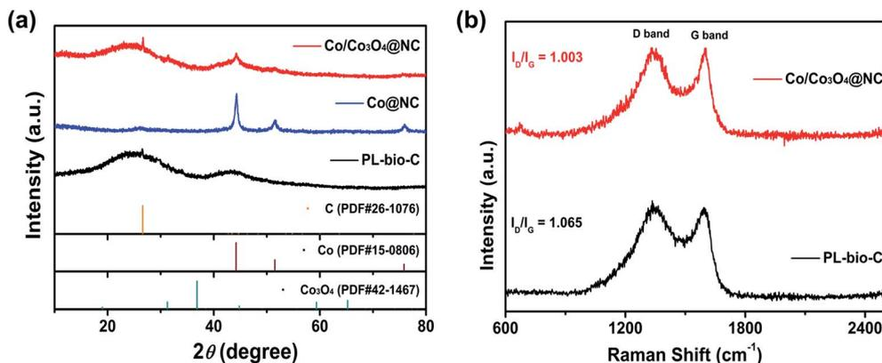
Fig. 4 (a) PXRD patterns of PL-bio-C, Co@NC, and Co/Co<sub>3</sub>O<sub>4</sub>@NC and (b) Raman spectra of PL-bio-C and Co/Co<sub>3</sub>O<sub>4</sub>@NC.
