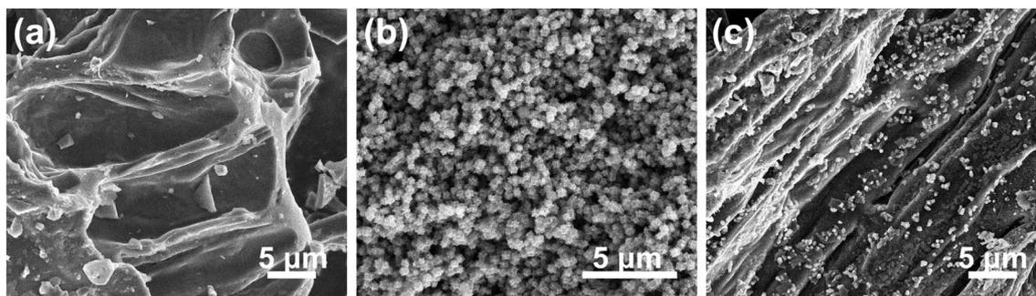
Fig. 2 Representative FE-SEM images of (a) PL-bio-C, (b) Co@NC, and (c) Co/Co<sub>3</sub>O<sub>4</sub>@NC.
