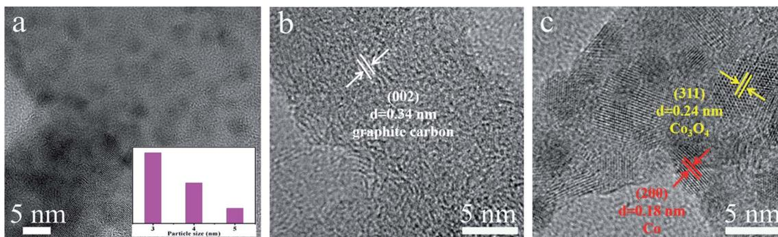
Fig. 3 (a) TEM image of the individual layer of Co/Co<sub>3</sub>O<sub>4</sub>@NC (inset shows the particle size distribution of Co/Co<sub>3</sub>O<sub>4</sub>@NC). Lattice fringe images of (b) graphitic carbon and (c) Co and Co<sub>3</sub>O<sub>4</sub> taken from the rectangular region, as obtained from the high-resolution TEM of Co/Co<sub>3</sub>O<sub>4</sub>@NC.
