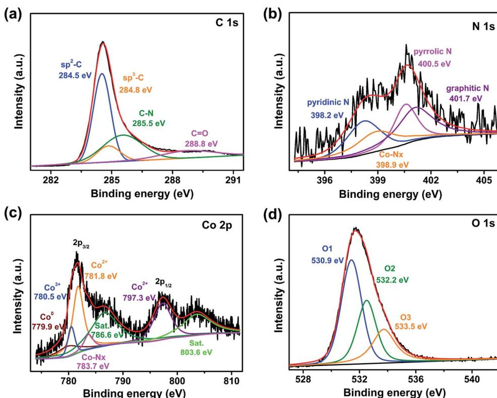
Fig. 5 High-resolution XPS curves of the (a) C 1s, (b) N 1s, (c) Co 2p, and (d) O 1s core levels for Co/Co<sub>3</sub>O<sub>4</sub>@NC.
