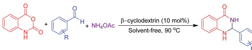
Scheme 2 One-pot three-component synthesis of 2,3-dihydroquinazolin-4(1 H )-one.
