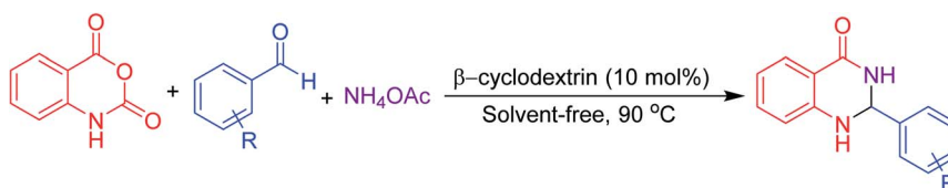
Scheme 2 One-pot three-component synthesis of 2,3-dihydroquinazolin-4(1 H )-one.
