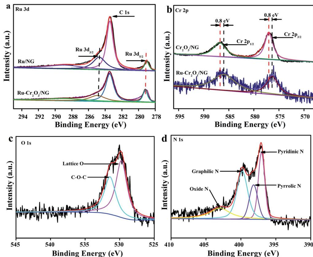
Fig. 3 Ru 3d (a), Cr 2p (b), O 1s (c) and N 1s (d) XPS of Ru-Cr<sub>2</sub>O<sub>3</sub>/NG.
