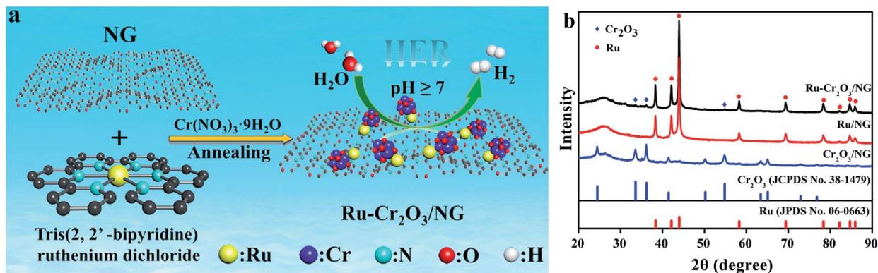
Fig. 1 Schematic illustration of the fabrication of Ru-Cr<sub>2</sub>O<sub>3</sub>/NG (a), XRD pattern of Ru-Cr<sub>2</sub>O<sub>3</sub>/NG, Ru/NG and Cr<sub>2</sub>O<sub>3</sub>/NG(b).
