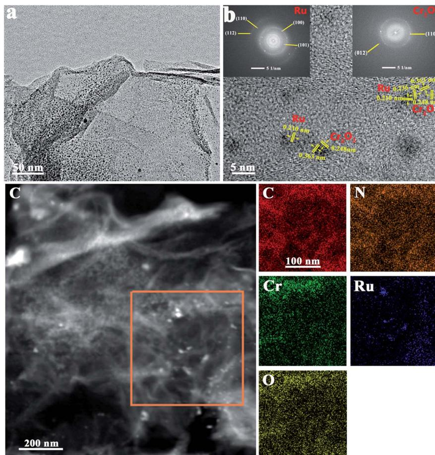
Fig. 2 TEM (a), HRTEM (b), STEM (c) images of Ru-Cr<sub>2</sub>O<sub>3</sub>/NG, and the corresponding elemental mapping of C, N, Cr, Ru and O. The insets in (b) are the FFT images of Ru and Cr<sub>2</sub>O<sub>3</sub>.
