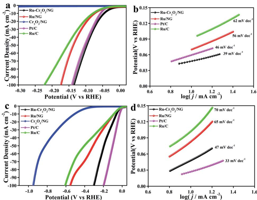
Fig. 4 Electrochemical HER activity of catalysts in alkaline (a and b) and neutral (c and d) medium. LSV curves (a and c), Tafel plots (b and d), Catalyst loading:  $0.15 \text{ mg Ru cm}^{-2}$  on GCE, scan rate:  $1 \text{ mV s}^{-1}$ .
