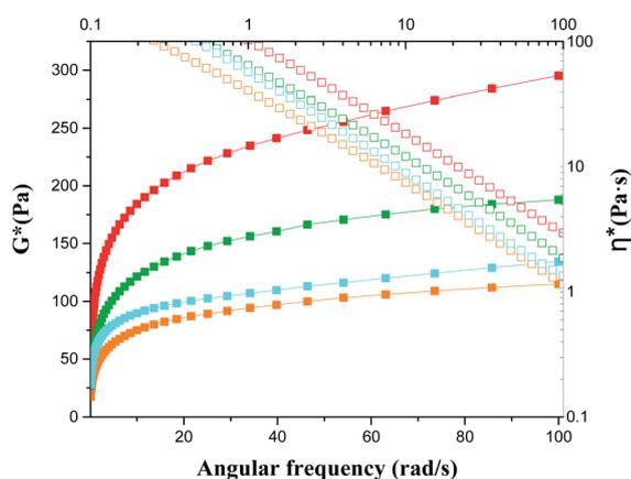
Fig. 8 Frequency dependent of  $G^*$  and  $\eta^*$  of P5–P8 (solid for  $G^*$ ; open for  $\eta^*$ ; orange for P5; red for P6; olive for P7; blue for P8).
