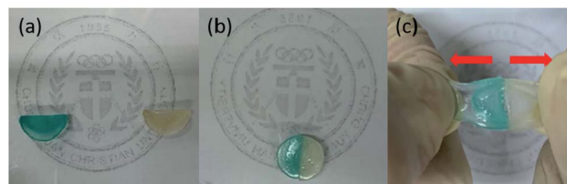
Fig. 3 Photographs of self-healing testing of damaged and healed P6 hydrogel.
