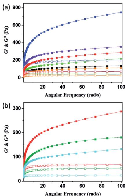
Fig. 7 Frequency dependent ( $\omega = 0.1$ – $100 \text{ rad s}^{-1}$ ) of rheology measurement of (a) P1–P6 and (b) P6–P8 hydrogels (solid for  $G'$  and open for  $G''$ ; black for P1; green for P2; violet for P3; indigo for P4; orange for P5; red for P6; olive for P7; blue for P8).
