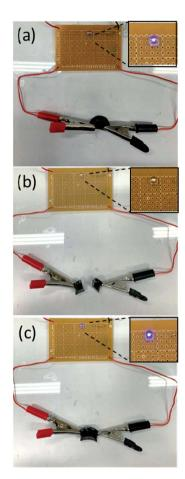
Fig. 11 Demonstration of a cutting and healing process for the P7 hydrogel connected in a circuit with a LED lamp. (a) Original sample, (b) cut sample and (c) self-healing sample.
