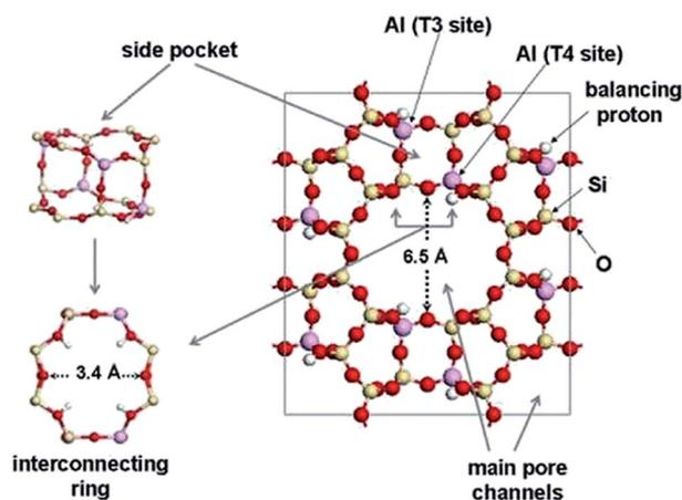
Fig. 4 The mordenite zeolite pore structure and dimensions.
