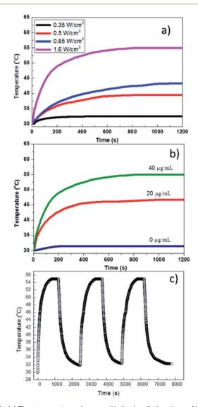
Fig. 7 (a) The temperature change with the irradiation time of hollow Au colloidal solution (40 μg mL<sup>-1</sup> concentration) under different power densities of the laser in the range from 0.35 to 1.6 W cm<sup>-2</sup>. (b) The temperature change with different concentrations of Au under 808 nm laser irradiation at the power density of 1.6  $\rm W \ cm^{-2}$ . (c) The stable photo-thermal conversion after three times irradiation under high power density of laser up to 1.6 W cm<sup>-2</sup>.
