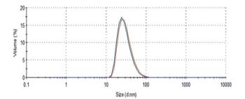
Fig. 4 DLS spectra of PMAO coated hollow Au nanostructure in water under different NaCl concentrations: 200 mM (blue), 250 mM (green) and 280 mM (red).
