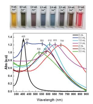
Fig. 5 UV-vis spectra of hollow gold samples synthesized with different volumes of HAuCl<sub>4</sub> solution (0, 0.5, 1.0, 1.5, 2.0, 2.5 and 3.5 mL) and the corresponding photos of their solution.
