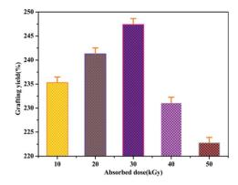
Fig. 7 Grafting yield of MCC-q-AM under different absorbed doses.
