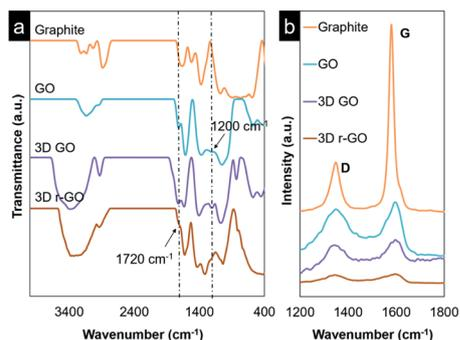
Fig. 3 (a) FT-IR spectra of graphite, graphene oxide, 3D hollow graphene and reduced 3D hollow graphene. The emergence of absorption peaks at 1720 cm<sup>-1</sup> and 1200 cm<sup>-1</sup> indicates the oxidation of graphite; upon reduction, the peaks disappear. (b) Raman spectra of graphite, graphene oxide, 3D hollow graphene and reduced 3D hollow graphene.
