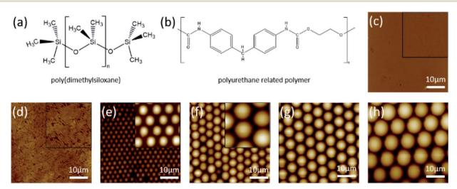
Fig. 2 (a and b) The chemical structures of two different polymers used to prepare the microlens arrays; (a) poly(dimethylsiloxane) and (b) polyurethane-related polymer. (c-h) Atomic force microscope images of (c) a flat surface without a physical structure and microlens arrays having diameters of (d) 0.5 μm, (e) 3 μm, (f) 5 μm, (g) 7 μm, and (h) 10 μm, respectively. The scanning dimension of insets was 10 μm by 10 μm.
