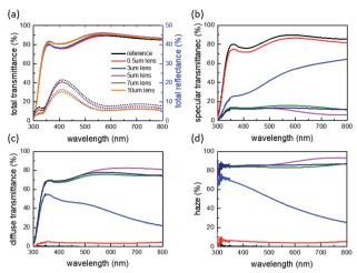
Fig. 5 (a) Total transmittance (solid line), total reflectance (dashed line), (b) specular transmittance, (c) diffuse transmittance, and (d) haze of microlens arrays with different sizes from 0.5 to  $10~\mu m$ .
