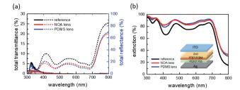
Fig. 4 (a) Total transmittance (solid line), total reflectance (dashed line), and (b) extinction of material stacks for organic photovoltaics in the absence and presence of a microlens array. The inset represents the materials and architecture of material stacks.
