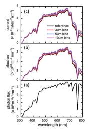
Fig. 8 (a) Photon flux of solar spectrum (AM 1.5 G), and the estimated (b) electron and (c) current generation of materials stacks for PTB7:PCBM organic photovoltaics in the absence and presence of microlens arrays with sizes 3  $\mu$ m, 5  $\mu$ m, and 10  $\mu$ m.
