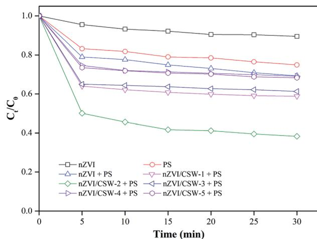
Fig. 3 Effect of different systems on MO degradation [PS] = 1 mM, [nZVI/CSW-1] = 1.25 g L<sup>-1</sup>, [nZVI/CSW-2] = 0.5 g L<sup>-1</sup>, [nZVI/CSW-3] = 0.25 g L<sup>-1</sup>, [nZVI/CSW-4] = 0.125 g L<sup>-1</sup>, [nZVI/CSW-5] = 0.1 g L<sup>-1</sup>, [nZVI] = 0.0625 g L<sup>-1</sup>, T = 20 ± 1 °C.
