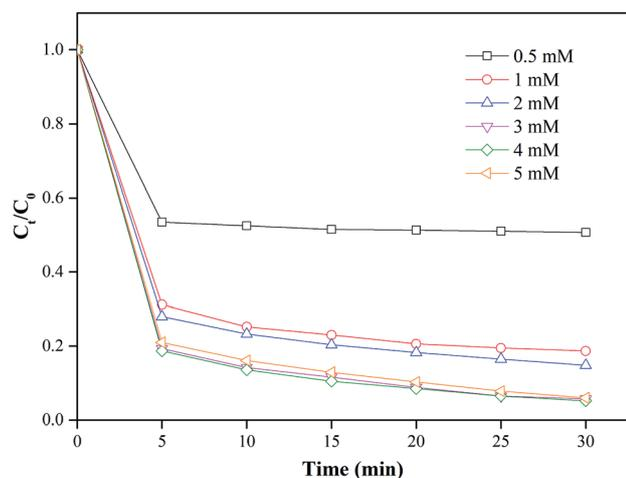
Fig. 5 Effect of PS addition on MO degradation, conditions: [MO] = 20 mg L<sup>-1</sup>, [nZVI/CSW-2] = 1.1 g L<sup>-1</sup>, [PS] = 0.5, 1, 2, 3, 4, 5 mM, T = 20 ± 1 °C.
