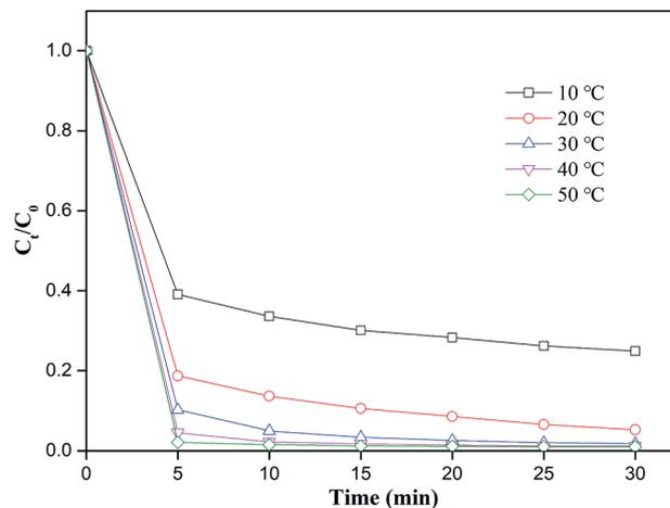
Fig. 6 Effect of temperature on MO removal efficiency, conditions: [MO] = 20 mg L<sup>-1</sup>, [PS] = 4 mM, [nZVI/CSW-2] = 1.1 g L<sup>-1</sup>, T = 10, 20, 30, 40, 50 °C respectively.
