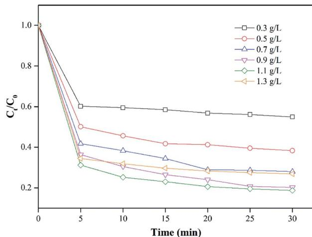
Fig. 4 Effect of nZVI/CSW-2 addition on MO degradation [MO] = 20 mg L<sup>-1</sup>, [PS] = 1 mM, [nZVI/CSW-2] = 0.3, 0.5, 0.7, 0.9, 1.1, 1.3 g L<sup>-1</sup>, T = 20 ± 1 °C.
