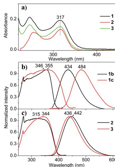
Fig. 2 Optical properties of THPs 1–3. (a) Absorption spectra of THPs 1–3 in cyclohexane solutions ( $1.0 \times 10^{-5}$  M). (b) and (c) Excitation (left) and emission (right) (excited at emission peak marked in the left excitation spectra) spectra of 1b, 1c, 2 and 3, respectively.
