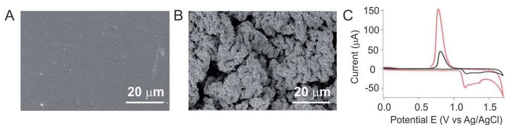
Fig. 2 We characterized both planar and wrinkled electrode using scanning electron microscopy and electrochemical techniques. (A) The planar gold film is smooth and uniform; (B) in contrast, after shrinking, the film exhibits a complex, hierarchically wrinkled structure (see Fig. S2† the greater magnification SEM for wrinkled electrode); (C) as expected, wrinkled gold film exhibits a 5.5-fold in surface area (red) of that observed for smooth gold film (black), which is in good accordance to our previous report. 20
