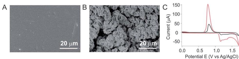
Fig. 2 We characterized both planar and wrinkled electrode using scanning electron microscopy and electrochemical techniques. (A) The planar gold film is smooth and uniform; (B) in contrast, after shrinking, the film exhibits a complex, hierarchically wrinkled structure (see Fig. S2† the greater magnified SEM for wrinkled electrode); (C) as expected, wrinkled gold film exhibits a 5.5-fold in surface area (red) of that observed for smooth gold film (black), which is in good accordance to our previous report. 20
