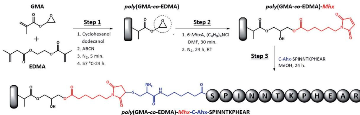
**Fig. 3** General scheme for the synthesis of the organic monolithic support of poly(GMA-co-EDMA) chemically modified with a peptide. Step 1: GMA-EDMA polymerization to obtain poly(GMA-co-EDMA). Step 2: grafting of poly(GMA-co-EDMA) with 6-maleimido-hexanoic acid to obtain poly(GMA-co-EDMA)-Mhx. Step 3: functionalization of poly(GMA-co-EDMA)-Mhx with a peptide containing a cysteine and 6-aminohexanoic residues and a sequence derived from L1-HPV protein.
