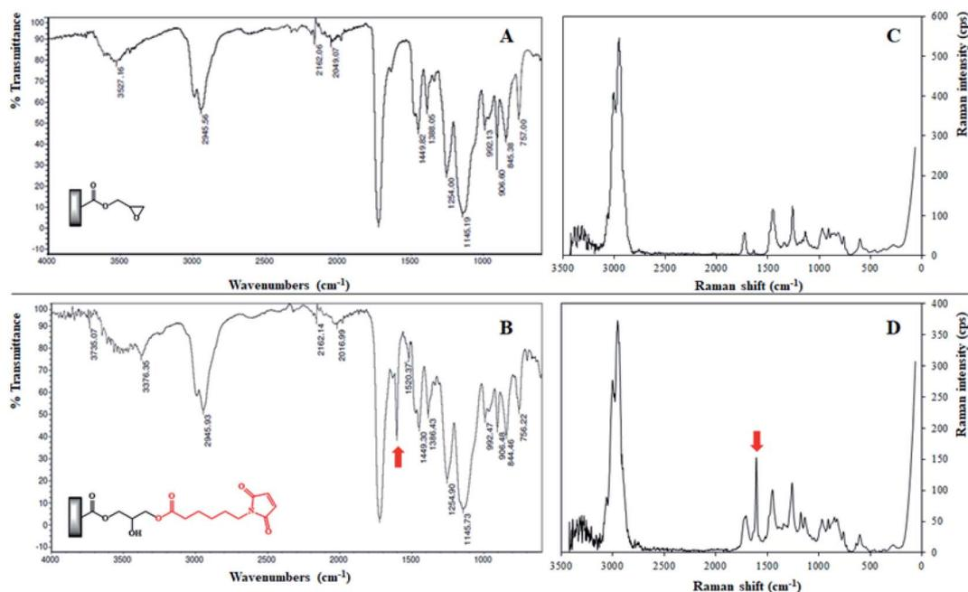
Fig. 5 Analysis of poly(GMA-*co*-EDMA) (top) and poly(GMA-*co*-EDMA)-*Mhx* (bottom) materials by means of FT-IR (A and B) and RAMAN (C and D). The red arrow indicates signals belonging to the maleimide group.
