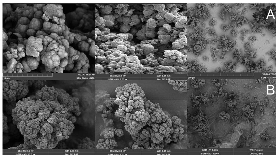
**Fig. 4** SEM images of monolithic materials: non-functionalized poly(GMA-co-EDMA) (A) and poly(GMA-co-EDMA)-Mhx (B).
