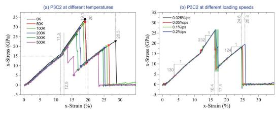
Fig. 4 Stress-strain curves of the P3C2 sample under tension, (a) at different temperatures with strain rate of 0.1% per ps, and (b) at different loading speeds with temperature of 300 K.
