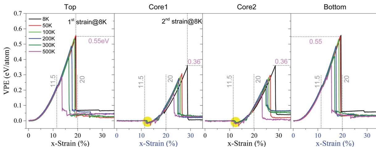
**Fig. 2** Histories of VPE per atom of the P3C2 sample under the strain rate of 0.1% per ps at different temperatures. Note that  $1^{\text{st}} \text{ strain} = 1^{\text{st}} \epsilon_c$  and  $2^{\text{nd}} \text{ strain} = 2^{\text{nd}} \epsilon_c$ .
