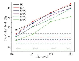
Fig. 10 The 2<sup>nd</sup> critical strains of sandwich carbon networks with different  $R_{L \text{ layer}}$  under the uniaxial tensile load at the strain rate of 0.1% per ps under different temperatures. The critical strains of the carbon network and pristine graphene under the same temperature are given with the same color, while the former is plotted with solid lines with symbols and the latter is drawn with broken lines.
