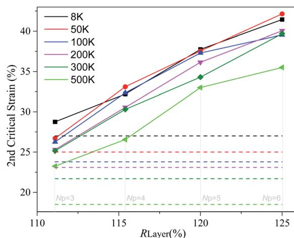
Fig. 10 The 2<sup>nd</sup> critical strains of sandwich carbon networks with different  $R_{\text{L layer}}$  under the uniaxial tensile load at the strain rate of 0.1% per ps under different temperatures. The critical strains of the carbon network and pristine graphene under the same temperature are given with the same color, while the former is plotted with solid lines with symbols and the latter is drawn with broken lines.
