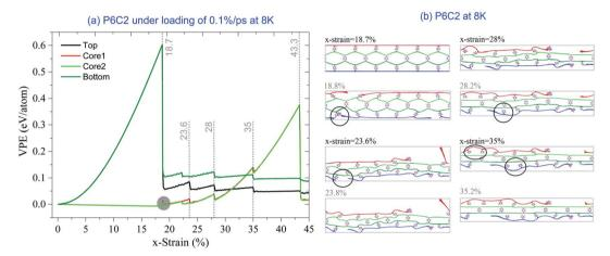
VPE curves of P6C2 under the loading speed of 0.1% per ps at 8 K. (a) VPE, (b) snapshots.
