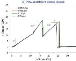
Fig. 6 Stress-strain curves of the P3C3 sample under tension. (a) At different temperatures at the strain rate of 0.1% per ps. (b) at different loading speeds with a temperature of 300 K.
