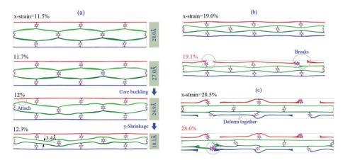
Fig. 3 Typical snapshots of the P3C2 sample under the strain rate of 0.1% per ps at 8 K. (a) The sample buckles with a sharply decreasing height when the x-strain is between 11.7% and 12.3%, (b) top layer breaks at x-strain = 19.1%, and (c) core 2 breaks when x-strain = 28.6%.
