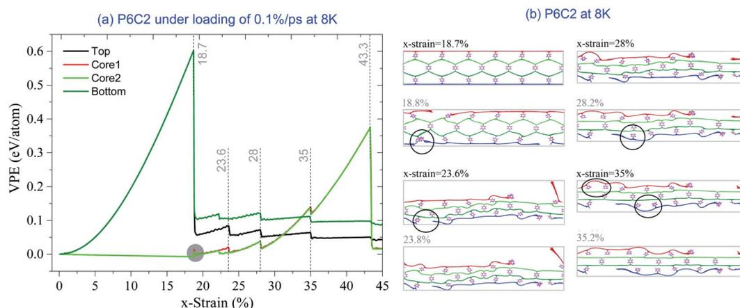
Fig. 9 VPE curves of P6C2 under the loading speed of 0.1% per ps at 8 K. (a) VPE, (b) snapshots.
