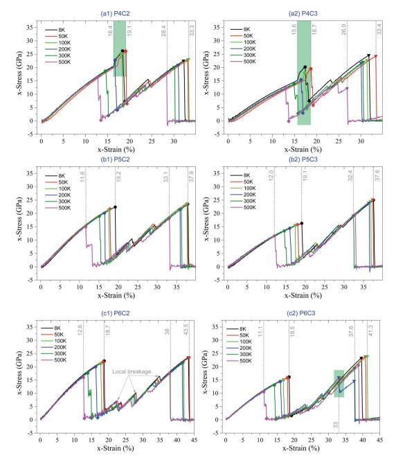
Fig. 7 Stress-strain curves of the samples under loading speed of 0.1% per ps at different temperatures. (a) P4C2 and P4C3, (b) P5C2 and P5C3, and (c) P6C2 and P6C3.
