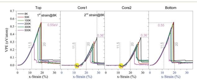
Fig. 2 Histories of VPE per atom of the P3C2 sample under the strain rate of 0.1% per ps at different temperatures. Note that  $1^{st}$  strain  $= 1^{st}$   $\epsilon_c$  and  $2^{nd}$  strain  $= 2^{nd}$   $\epsilon_c$ .
