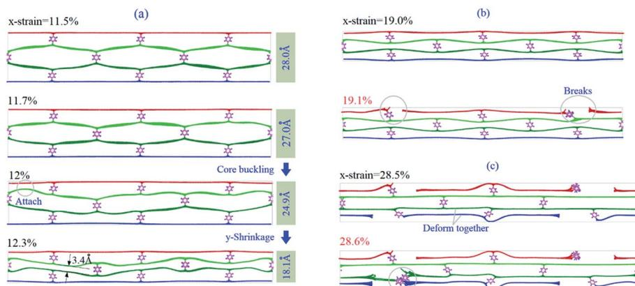
Fig. 3 Typical snapshots of the P3C2 sample under the strain rate of 0.1% per ps at 8 K. (a) The sample buckles with a sharply decreasing height when the  $x$ -strain is between 11.7% and 12.3%, (b) top layer breaks at  $x$ -strain = 19.1%, and (c) core 2 breaks when  $x$ -strain = 28.6%.
