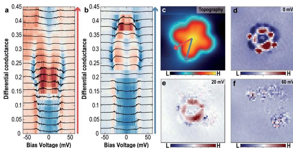
Fig. 4 The spatial variation of the tunnelling spectra of the trapped H<sub>2</sub> (a and b) evolution of the tunnelling spectra along the high symmetric lines of the VOPc molecule following red arrow (a) and blue arrow (b) as shown in (c). (c–f) Simultaneously obtained topographic image of the single O-up VOPc molecule (c) and *dI/dV* maps (d–f) with different bias voltages. Images size is 3 nm × 3 nm.
