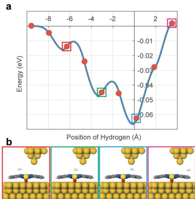
Fig. 3 (a) The energy potential of H<sub>2</sub> along the VOPc molecule. The distance is relative to the STM tip apex atom. (b) Graphical representations for selected points along the diffusion paths are shown.
