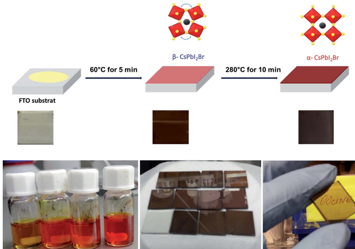
Fig. 1 Scheme showing the one spin-coating process of deposition of CsPbI<sub>2</sub>Br thin films and the visual image of the dark brown colored phase of CsPbI<sub>2</sub>Br film synthesized in this work.
