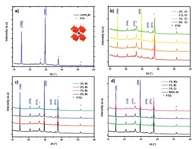
Fig. 2 XRD pattern of spin coated CsPbl<sub>2</sub>Br films with different additives: (a) CsPbl<sub>2</sub>Br with HI, (b) with different amounts of chloride, (c) with x% of bismuth, (d) XRD pattern of CsPbl<sub>2</sub>Br with different additives.
