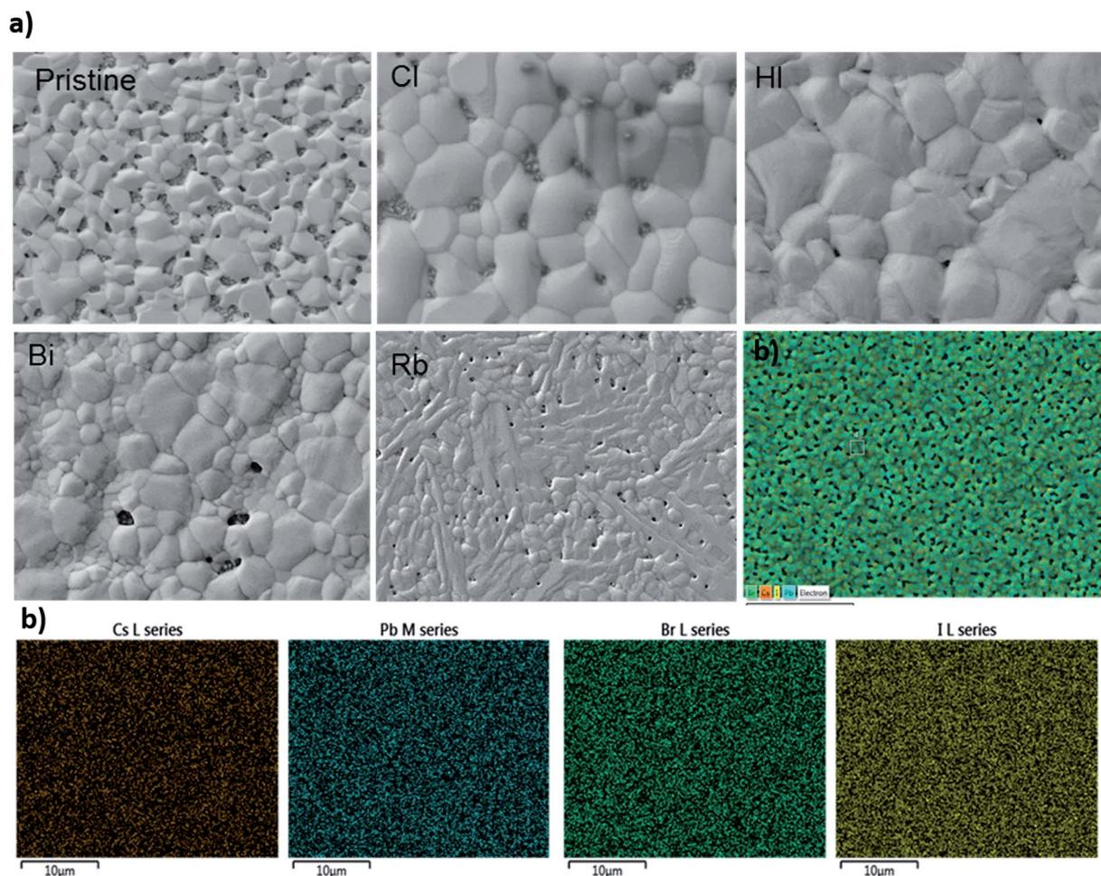
Fig. 4 (a) Top-view SEM images of the CsPbI<sub>2</sub>Br film with different additives (b) EDS mapping of CsPbI<sub>2</sub>Br with showing the map distribution of Cs, Pb, I and Br elements. EDS map confirms the uniform distribution of Cs, I and Br elements.
