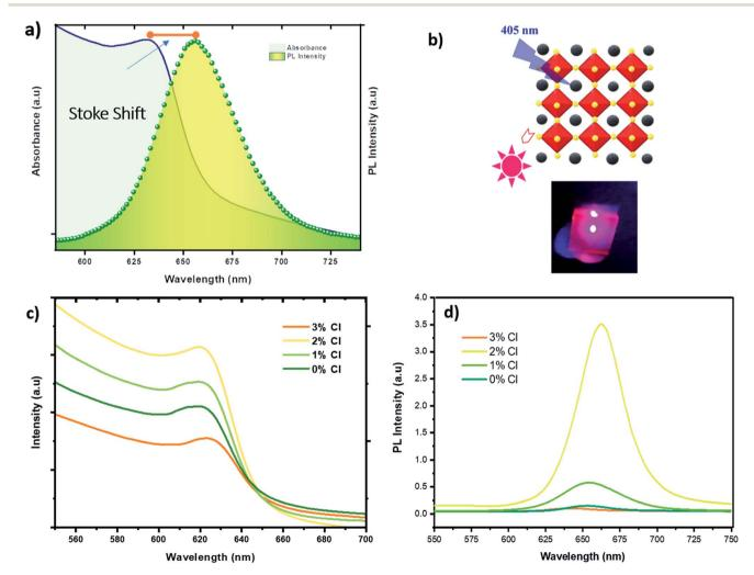
Fig. 6 (a) RT absorption and PL spectra of CsPbl<sub>2</sub>Br thin films deposited on FTO substrate (b) scheme of the cubic perovskite crystal structure of CsPbl<sub>2</sub>Br with a photograph of the Red PL emission (c) absorbance spectra of undoped and Cl doped CsPbl<sub>2</sub>Br/FTO samples (d) PL spectra of undoped and Cl doped CsPbl<sub>2</sub>Br/FTO samples.
