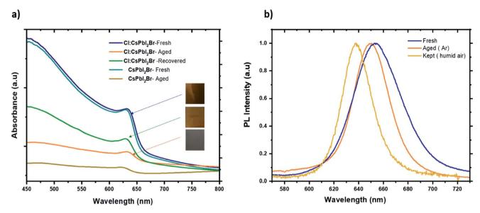
Fig. 9 (a) Absorbance spectrum of fresh, aged, and recovered Cl:CsPbl<sub>2</sub>Br thin film. (b) PL spectra of fresh, aged samples of Cl:CsPbl<sub>2</sub>Br films kept in argon and in a humid air.
