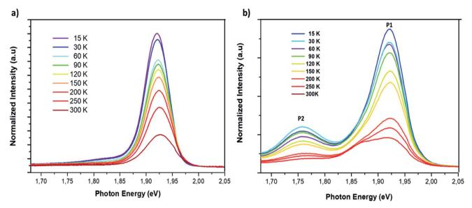
Fig. 7 Temperature dependent photoluminescence spectrum of CsPbl<sub>2</sub>Br (a) and 2% Cl doped CsPbl<sub>2</sub>Br (b) with excitation by a 405 nm laser beam
