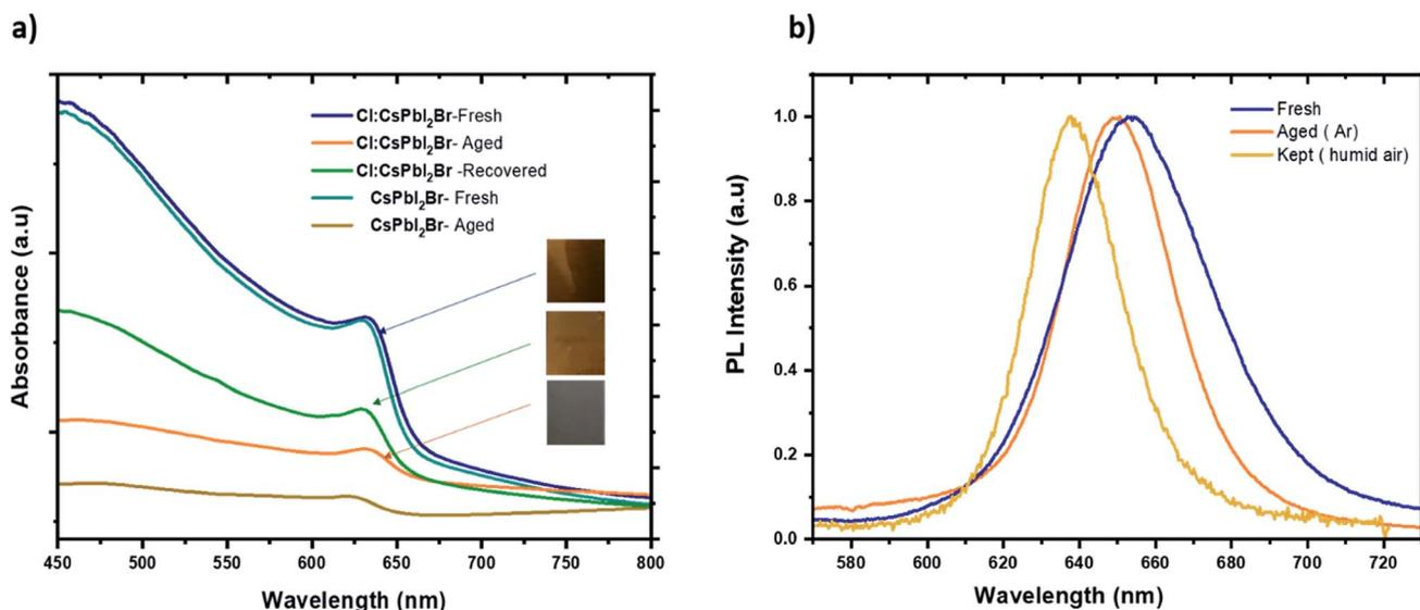
Fig. 9 (a) Absorbance spectrum of fresh, aged, and recovered Cl:CsPbI<sub>2</sub>Br thin film. (b) PL spectra of fresh, aged samples of Cl:CsPbI<sub>2</sub>Br films kept in argon and in a humid air.
