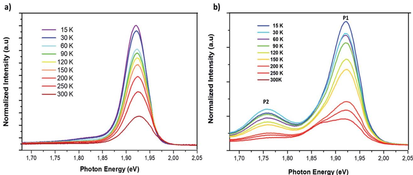
Fig. 7 Temperature dependent photoluminescence spectrum of CsPbI<sub>2</sub>Br (a) and 2% Cl doped CsPbI<sub>2</sub>Br (b) with excitation by a 405 nm laser beam.
