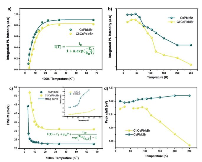
Fig. 8 (a and b) Integrated PL intensity as a function of temperature of the  $CsPbl_2Br$  and 2% Cl doped  $CsPbl_2Br$  thin films. The integrated PL intensity was normalized to the initial intensity. (c) Temperature dependent Gauss-fitted full widths at half maximum (FWHMs) and (d) position of the  $CsPbl_2Br$  and 2% Cl doped  $CsPbl_2Br$  thin films.
