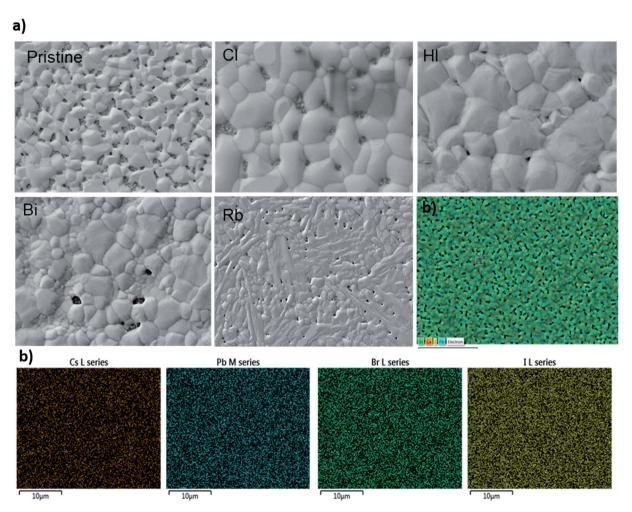
Fig. 4 (a) Top-view SEM images of the CsPbl<sub>2</sub>Br film with different additives (b) EdS mapping of CsPbl<sub>2</sub>Br with showing the map distribution of Cs, Pb, I and Br elements. EDS map confirms the uniform distribution of Cs, I and Br elements.
