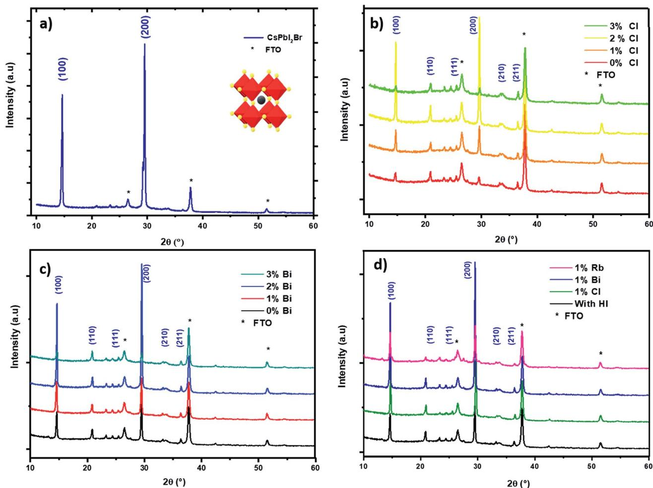
Fig. 2 XRD pattern of spin coated CsPbI<sub>2</sub>Br films with different additives: (a) CsPbI<sub>2</sub>Br with HI, (b) with different amounts of chloride, (c) with x% of bismuth, (d) XRD pattern of CsPbI<sub>2</sub>Br with different additives.
