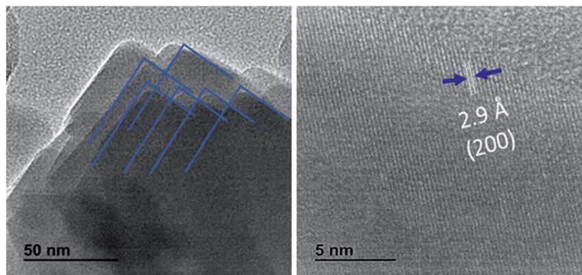
Fig. 5 HRTEM Images of CsPbI<sub>2</sub>Br films. The interplanar spacing of 0.29 nm corresponding to the (200) plane of 3D perovskites was observed.
