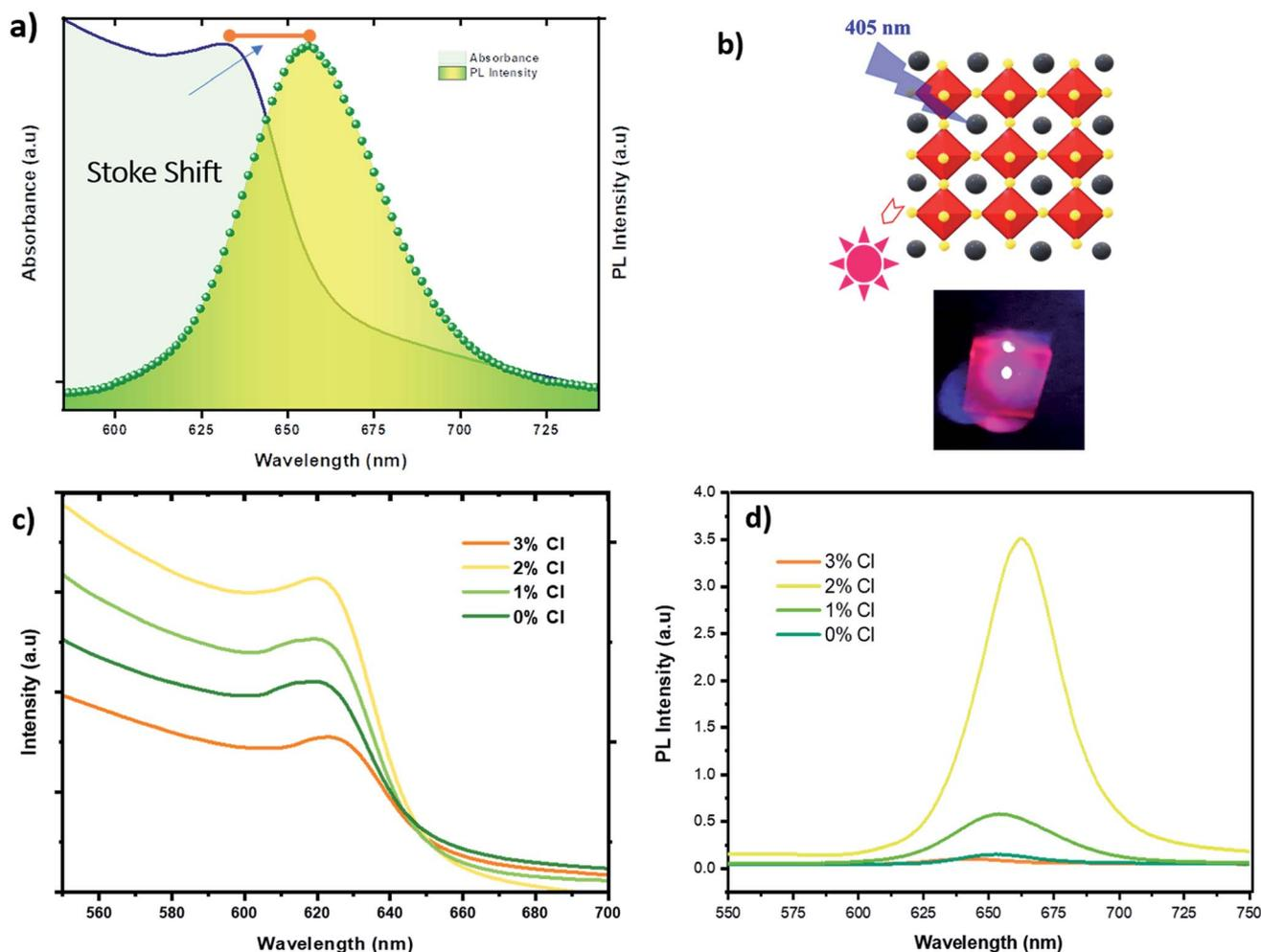
Fig. 6 (a) RT absorption and PL spectra of CsPbI<sub>2</sub>Br thin films deposited on FTO substrate (b) scheme of the cubic perovskite crystal structure of CsPbI<sub>2</sub>Br with a photograph of the Red PL emission (c) absorbance spectra of undoped and Cl doped CsPbI<sub>2</sub>Br/FTO samples (d) PL spectra of undoped and Cl doped CsPbI<sub>2</sub>Br/FTO samples.
