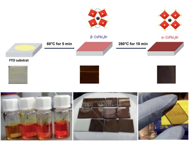
Fig. 1 Scheme showing the one spin-coating process of deposition of CsPBI<sub>2</sub>Br thin films and the visual image of the dark brown colored phase of CsPbI<sub>2</sub>Br film synthesized in this work.
