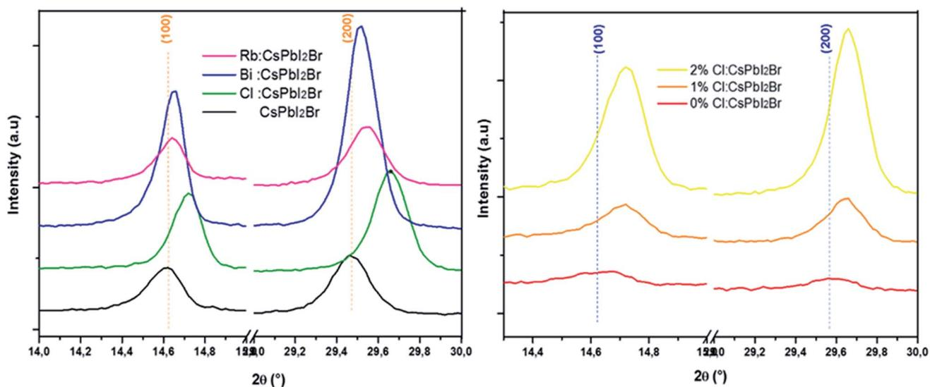
Fig. 3 Shift of (100) and (200) XRD peaks of doped CsPbI<sub>2</sub>Br perovskite.
