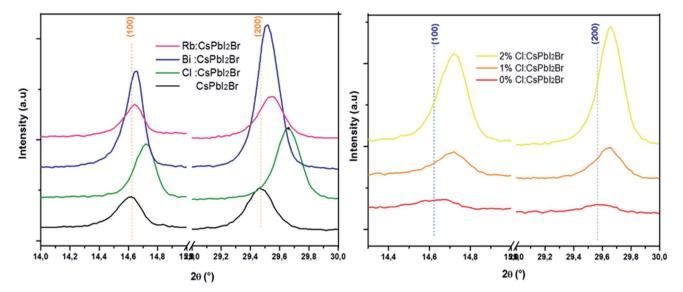
Fig. 3 Shift of (100) and (200) XRD peaks of doped CsPbl<sub>2</sub>Br perovskite.
