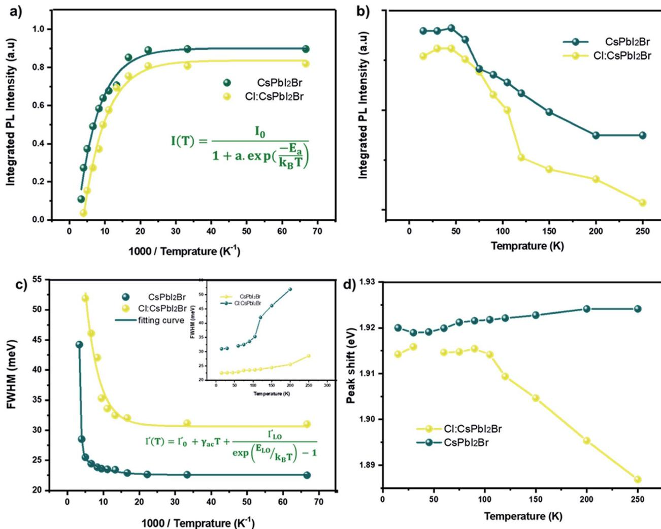
Fig. 8 (a and b) Integrated PL intensity as a function of temperature of the CsPbI<sub>2</sub>Br and 2% Cl doped CsPbI<sub>2</sub>Br thin films. The integrated PL intensity was normalized to the initial intensity. (c) Temperature dependent Gauss-fitted full widths at half maximum (FWHMs) and (d) position of the CsPbI<sub>2</sub>Br and 2% Cl doped CsPbI<sub>2</sub>Br thin films.
