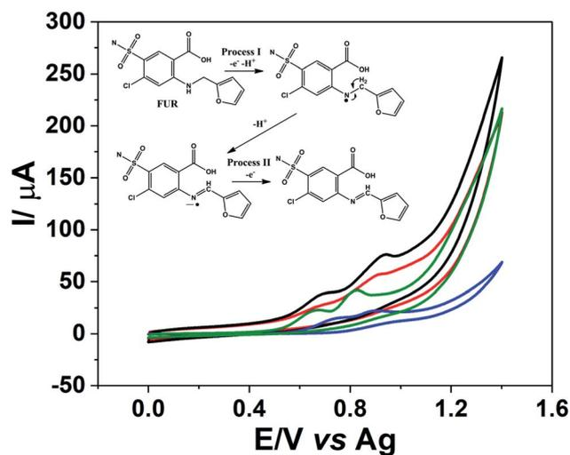
Fig. 6 CVs recorded using different carbon electrodes: (red line) non-treated PDE, (black line) CO<sub>2</sub> laser-treated PDE, (blue line) commercial screen-printed carbon electrode, (green line) commercial screen-printed graphene electrode in a solution of 1 mmol L<sup>-1</sup> FUR in 0.1 mol L<sup>-1</sup> PBS (pH = 6.8). Inset: schematic representation of FUR oxidation mechanism. Scan rate: 10 mV s<sup>-1</sup>.
