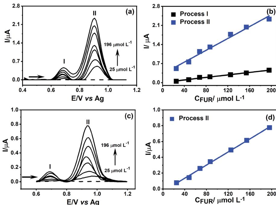
Fig. 7 DPVs recorded using (a) CO<sub>2</sub> laser-treated and (c) CO<sub>2</sub> non-treated PDEs in 0.1 mol L<sup>-1</sup> PBS (pH = 6.8) (dashed lines) containing 25, 48, 68, 87, 125, 154, and 196 μmol L<sup>-1</sup> FUR (solid lines), (b and d) calibration curves obtained from FUR measurements for both CO<sub>2</sub> laser-treated and non-treated PDEs, respectively. Parameters: scan rate: 20 mV s<sup>-1</sup>, amplitude: 50 mV, and step: 10 mV.
