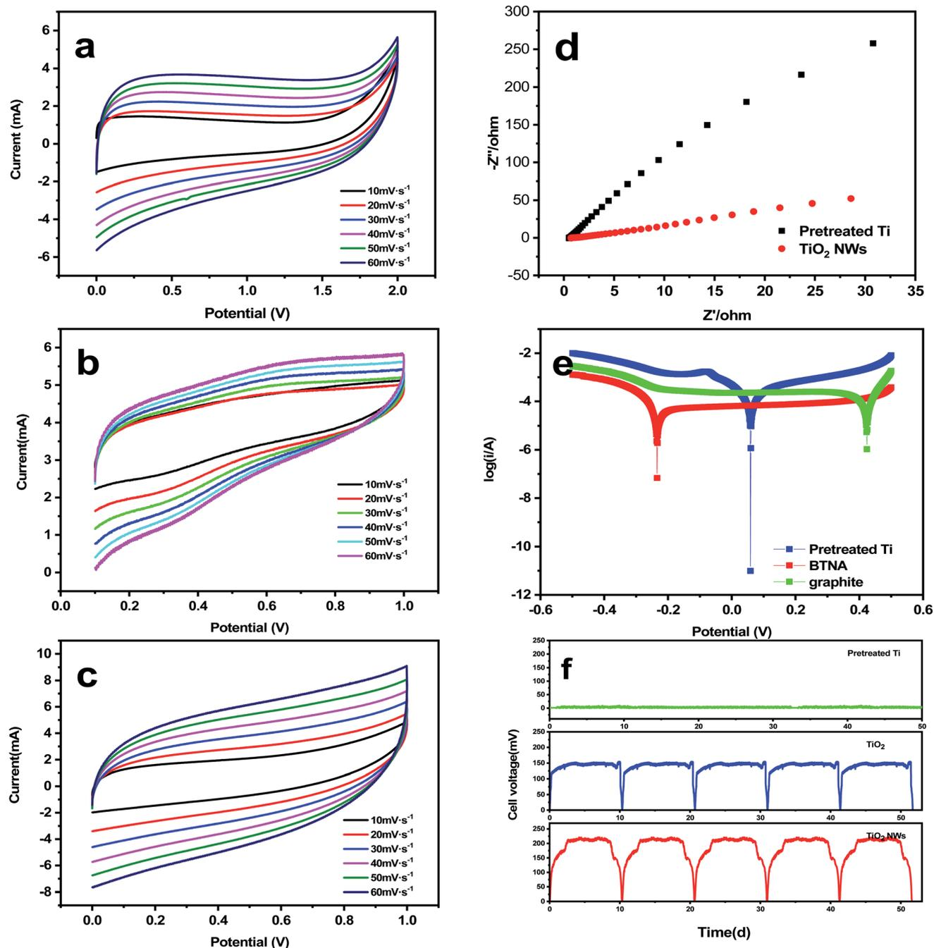
Fig. 2 Electrochemical tests in electrolyte. (a) CV curves of TiO<sub>2</sub> NWs electrode electrolyte in three-electrode mode. (b) CV curves of TiO<sub>2</sub> NWs anode in two-electrode mode. (c) CV curves of TiO<sub>2</sub> NWs cathode in two-electrode mode. (d) Nyquist plots of different electrodes and equivalent circuits used to fit the EIS data. (e) Tafel polarization curves of different electrode. (f) The cells voltage over time under external resistance.
