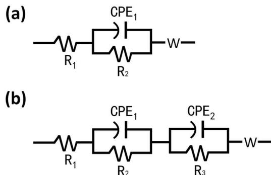
Fig. 3 Equivalent circuit models were used in the analysis of electrodes in MFCs (a) under the dark conditions (b) under illumination.
