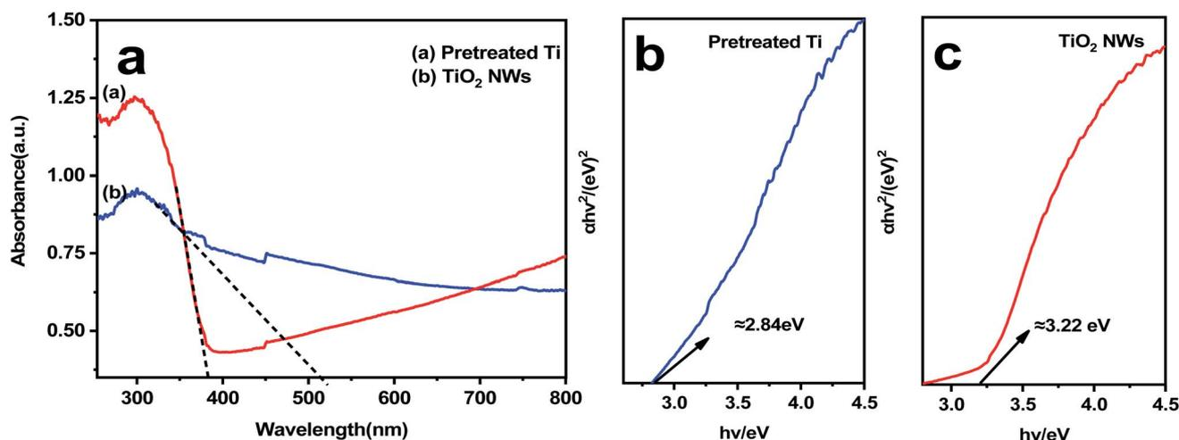
Fig. 4 (a) UV-visible light absorption DRS patterns, (b) calculated energy bandgap of pretreated titanium plates, (c) calculated energy bandgap of TiO<sub>2</sub> NWs.
