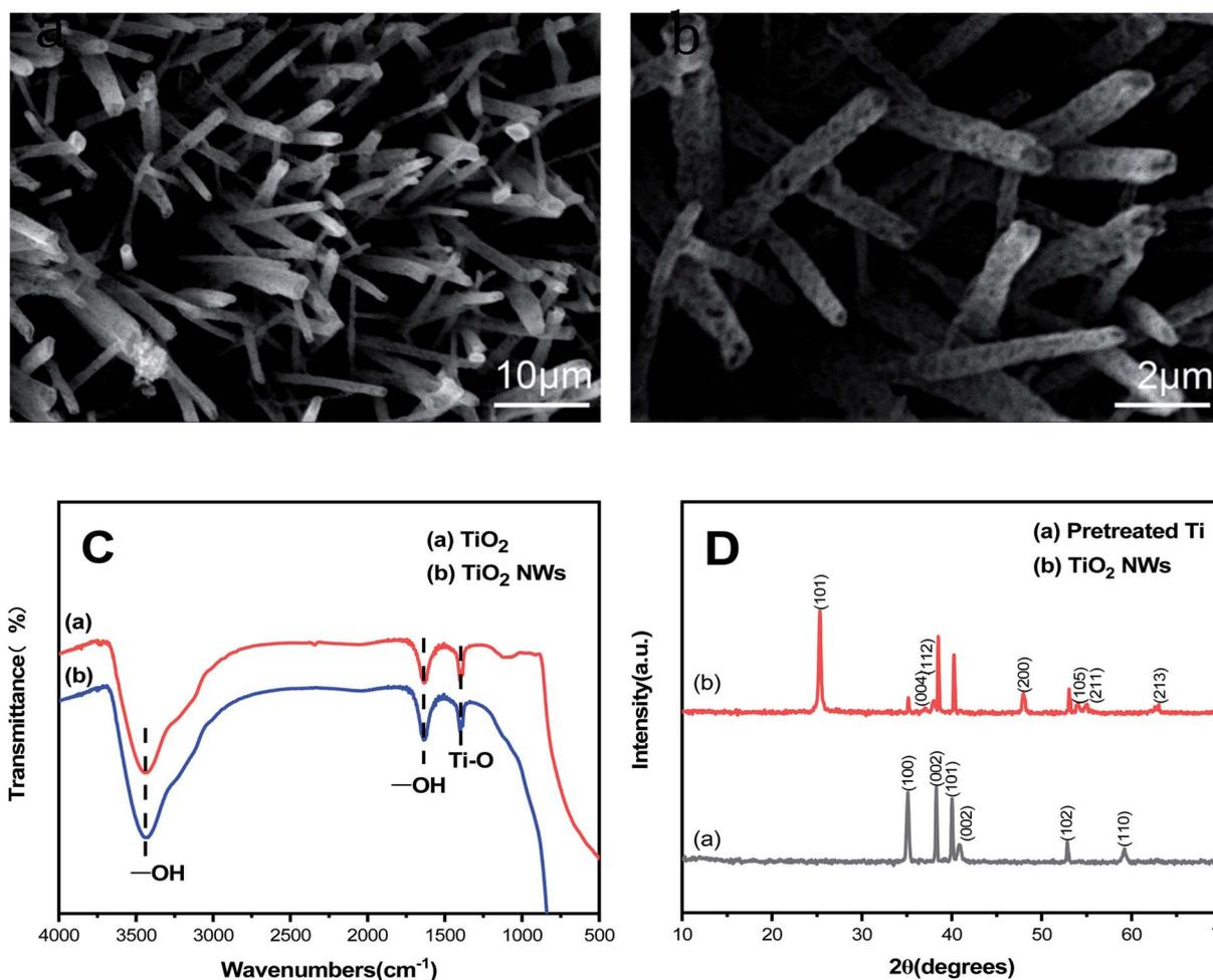
Fig. 1 (a and b) SEM image of the TiO<sub>2</sub> NWs electrode. (c) FTIR spectra of commercial titanium dioxide and TiO<sub>2</sub> NWs electrode. (d) XRD pattern after pretreatment.
