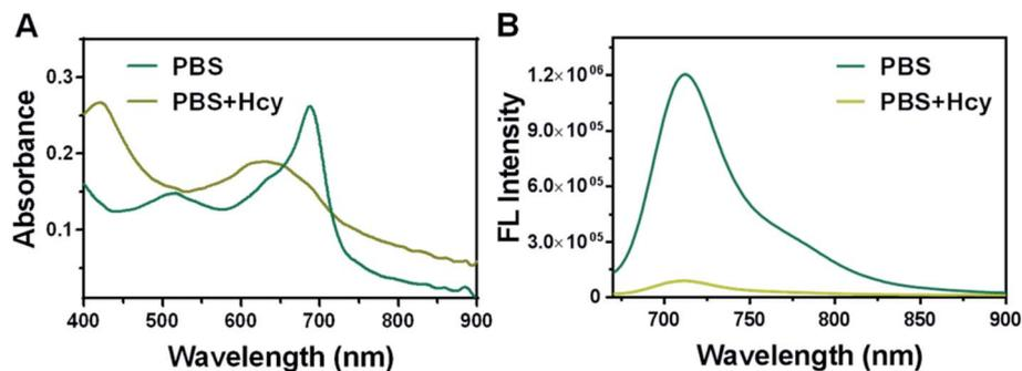
Fig. 1 (A) The UV/Vis spectrum of HSFP (10  $\mu$ M) toward 1 mM Hcy was measured in PBS/DMSO buffer (9/1, v/v, pH 7.4). (B) Fluorescence spectrum of HSFP (10  $\mu$ M) toward 1 mM Hcy was measured in PBS/DMSO buffer (9/1, v/v, pH 7.4),  $\lambda_{em}$  = 650 nm.
