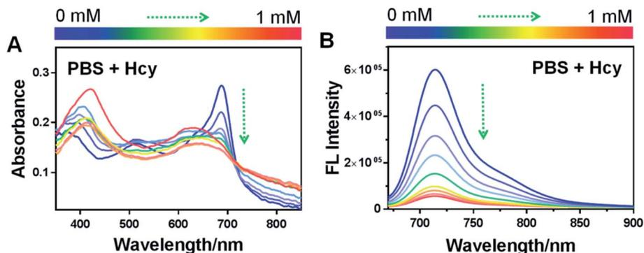
Fig. 3 (A) The UV/Vis spectrum of HSFP (10  $\mu\text{M}$ ) toward 0–1 mM Hcy were measured in PBS/DMSO buffer (9/1, v/v, pH 7.4). (B) Fluorescence spectrum of HSFP (10  $\mu\text{M}$ ) toward 0–1 mM Hcy were measured in PBS/DMSO buffer (9/1, v/v, pH 7.4),  $\lambda_{\text{em}} = 650 \text{ nm}$ .
