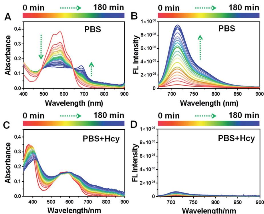
Fig. 2 The time-dependent UV/Vis spectrum (A) and fluorescence spectrum (B) of HSFP (10  $\mu$ M) in PBS were measured in PBS/DMSO buffer (9/1, v/v, pH 7.4). The time-dependent UV/Vis spectrum (C) and fluorescence spectrum (D) of HSFP (10  $\mu$ M) toward 1 mM Hcy were measured in PBS/DMSO buffer (9/1, v/v, pH 7.4).
