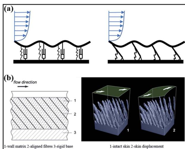
**Fig. 9** (a) Compliant wall models. Reproduced from ref. 103 with permission from Cambridge University Press, copyright 2019. (b) Compliant wall structure and the simulation for the deformation of dolphin skin along with shear stress. Reproduced from ref. 56 with permission from IOP Publishing Ltd, copyright 2006.
