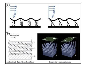
Fig. 9 (a) Compliant wall models. Reproduced from ref. 103 with permission from Cambridge University Press, copyright 2019. (b) Compliant wall structure and the simulation for the deformation of dolphin skin along with shear stress. Reproduced from ref. 56 with permission from IOP Publishing Ltd, copyright 2006.
