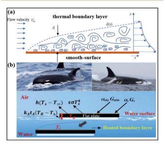
Fig. 10 (a) Schematic diagram of the thermal boundary layer over the wing. Reproduced from ref. 107 with permission from Elsevier Ltd, copyright 2017. (b) Schematic diagram of energy conservation in the heated boundary layer. Reproduced from ref. 108 with permission from Elsevier Ltd, copyright 2019.
