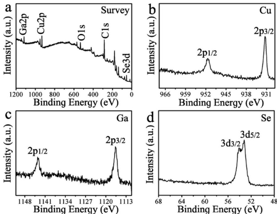
Fig. 3 XPS spectra of the as-prepared CuGaSe<sub>2</sub> plates. (a) Survey spectrum, (b) Cu 2p core level spectrum, (c) Ga 2p core level spectrum, and (d) Se 3d core level spectrum.
