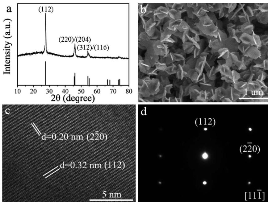
Fig. 1 (a) XRD pattern along with standard JCPDS no. 31-0456 for reference and (b) SEM image of the as-synthesized  $\text{CuGaSe}_2$  plates. (c) HRTEM image and (d) the corresponding SAED pattern of the  $\text{CuGaSe}_2$  plates.
