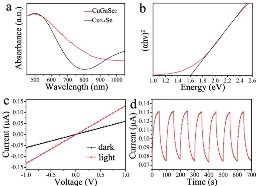
Fig. 7 (a) UV-vis-NIR absorption spectra of  $\text{Cu}_2-x\text{Se}$  and  $\text{CuGaSe}_2$  plates dispersed in toluene. (b) The linear extrapolations of plots of  $(\alpha h\nu)^2$  vs. photon energy. (c) Current versus voltage curves of the  $\text{CuGaSe}_2$  plates measured in dark and under xenon lamp illumination with a power intensity of  $6.5 \text{ mW cm}^{-2}$ , and (d) current versus time curves during ON and OFF cycles.
