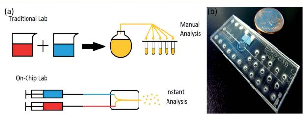
Fig. 2 (a) Lab-on-chip in comparison with traditional lab, (b) a microfluidic chip compare to a coin, adapted from ref. 41.
