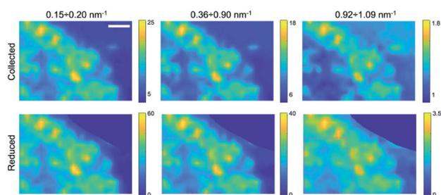
Fig. 3 SAXS maps in different  $q$ -ranges for the wet POPC sample. From left to right (in both rows):  $0.15 \div 0.20$ ,  $0.36 \div 0.90$ ,  $0.92 \div 1.09$  nm<sup>-1</sup>. Upper row: as collected data; lower row: reduced data; in the area delimited by the dotted line, corresponding to low POPC concentration, the contrast is visibly changing as a function of the chosen  $Q$ -range, compared to the surrounding regions. Scale bar: 1 mm.
