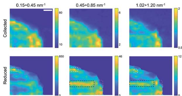
Fig. 4 SAXS maps in different  $Q$ -ranges for the dried POPC sample. From left to right (in both rows):  $0.15 \div 0.45$ ,  $0.45 \div 0.85$ ,  $1.02 \div 1.20$   $\text{nm}^{-1}$ . Upper row: as collected data; lower row: reduced data; in the areas delimited by dotted lines, the contrast is visibly changing as a function of the chosen  $Q$ -range. Scale bar: 1 mm.
