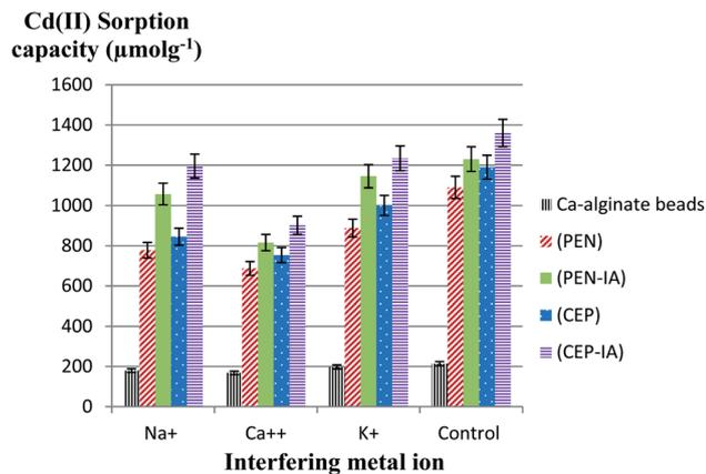
Fig. 12 Effect of metal ion interference on Cd(II) sorption capacity by free and immobilized fungal biomass in Ca-alginate beads. PEN: free *Penicillium chrysogenum*, PEN-IA: *Penicillium chrysogenum* immobilized in Ca-alginate beads, CEP: free *Cephalotheca foveolata*, CEP-IA: *Cephalotheca foveolata* immobilized in Ca-alginate beads.
