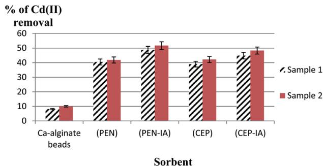
Fig. 14 Removal of Cd(II) from real wastewater samples by free and immobilized fungal biomass in Ca-alginate beads. PEN: free *Penicillium chrysogenum*, PEN-IA: *Penicillium chrysogenum* immobilized in Ca-alginate beads, CEP: free *Cephalotheca foveolata*, CEP-IA: *Cephalotheca foveolata* immobilized in Ca-alginate beads. Sample (1): wastewater collected from General Motors Factory in Giza, sample (2): wastewater collected from Egyptian Plastic and Electricity Factory in Cairo.
