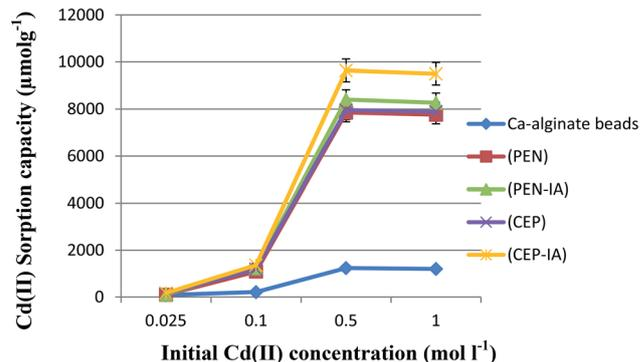
Fig. 10 Effect of different initial Cd(II) concentrations on Cd(II) sorption capacity by free and immobilized fungal biomass in Ca-alginate beads. PEN: free *Penicillium chrysogenum*, PEN-IA: *Penicillium chrysogenum* immobilized in Ca-alginate beads, CEP: free *Cephalotheca foveolata*, CEP-IA: *Cephalotheca foveolata* immobilized in Ca-alginate beads.
