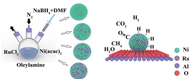
Scheme 1 Schematic of the preparation procedure of monodispersed NiRu NPs for CO<sub>2</sub> methanation.
