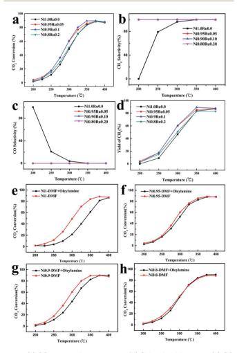
Fig. 3 (a) CO<sub>2</sub> conversion rate curve, (b) CH<sub>4</sub> selectivity curve, (c) CO selectivity curve, (d) CH<sub>4</sub> yield curve of NiRu/Al<sub>2</sub>O<sub>3</sub> at different temperatures. (e-h) The catalytic performance of CO<sub>2</sub> methanation  $Ni_xRu_{(1-x)}/\gamma$ -Al<sub>2</sub>O<sub>3</sub> prepared with different solutions of NaBH<sub>4</sub>.
