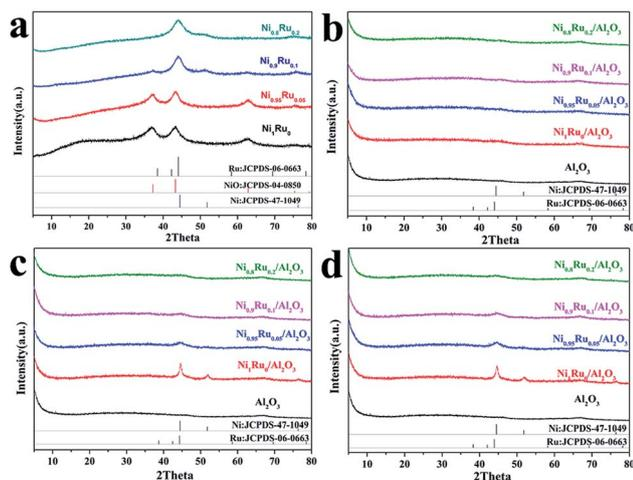
Fig. 2 XRD results of (a) NiRu NPs with Ar treatment at 300 °C, (b) NiRu/Al<sub>2</sub>O<sub>3</sub>, (c) and (d) NiRu/Al<sub>2</sub>O<sub>3</sub> after H<sub>2</sub> reduction and after the catalytic performance test.
