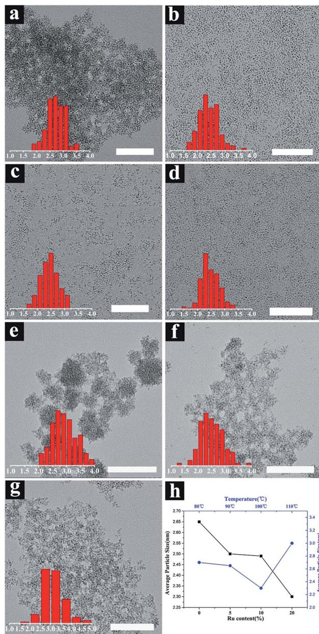
Fig. 1 TEM results of (a–d) Ni<sub>1</sub>Ru<sub>0</sub>, Ni<sub>0.95</sub>Ru<sub>0.05</sub>, Ni<sub>0.9</sub>Ru<sub>0.1</sub> and Ni<sub>0.8</sub>Ru<sub>0.2</sub> nanoparticles at a synthetic temperature of 90 °C (scan bar: 100 nm). (d–g) Ni<sub>1</sub>Ru<sub>0</sub> nanoparticles at synthesis temperatures of 80, 100 and 110 °C. (h) Particle size of Ni<sub>1</sub>Ru<sub>0</sub> nanoparticles at different synthesis temperatures.
