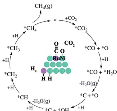
Fig. 5 CO<sub>2</sub> methanation scheme on NiRu/Al<sub>2</sub>O<sub>3</sub>.
