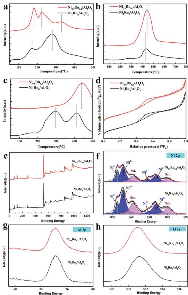
Fig. 4 (a) H<sub>2</sub>-TPR, (b) H<sub>2</sub>-TPD, (c) CO<sub>2</sub>-TPD profile of NiRu/Al<sub>2</sub>O<sub>3</sub>, (d) N<sub>2</sub> adsorption–desorption isotherms of NiRu/Al<sub>2</sub>O<sub>3</sub>, (e) Survey scan, (f) High-resolution Ni 2p spectra, (g) High-resolution Al 2p spectra, (h) High-resolution O 1s spectra.
