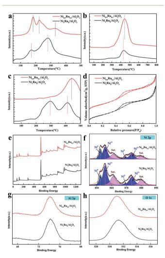
Fig. 4 (a)  $\rm H_2$ -TPR, (b)  $\rm H_2$ -TPD, (c)  $\rm CO_2$ -TPD profile of NiRu/Al $_2\rm O_3$ , (d)  $\rm N_2$  adsorption—desorption isotherms of NiRu/Al $_2\rm O_3$ . (e) Survey scan. (f) High-resolution Ni 2p spectra. (g) High-resolution Al 2p spectra. (h) High-resolution O 1s spectra.
