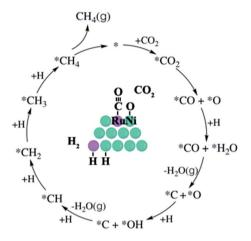
Fig. 5 CO<sub>2</sub> methanation scheme on NiRu/Al<sub>2</sub>O<sub>3</sub>.
