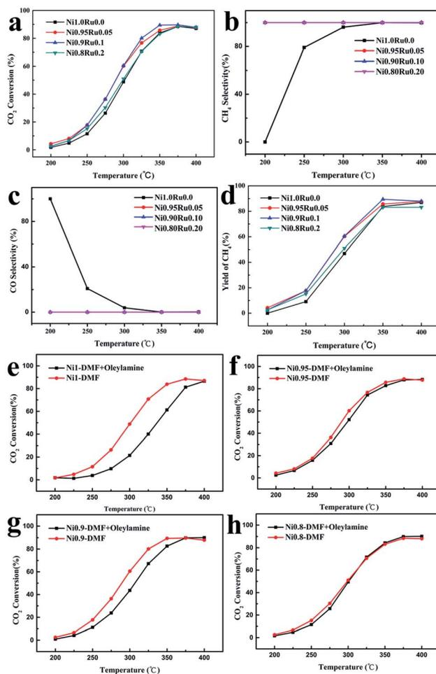
Fig. 3 (a) CO<sub>2</sub> conversion rate curve, (b) CH<sub>4</sub> selectivity curve, (c) CO selectivity curve, (d) CH<sub>4</sub> yield curve of NiRu/Al<sub>2</sub>O<sub>3</sub> at different temperatures. (e–h) The catalytic performance of CO<sub>2</sub> methanation Ni<sub>x</sub>Ru<sub>(1-x)</sub>γ-Al<sub>2</sub>O<sub>3</sub> prepared with different solutions of NaBH<sub>4</sub>.
