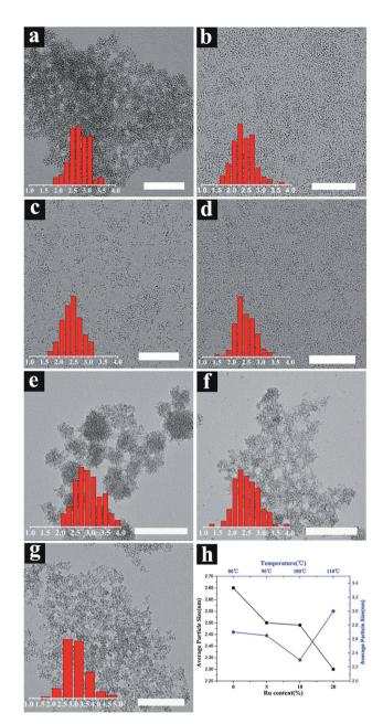
Fig. 1 TEM results of (a–d)  $Ni_1Ru_0$ ,  $Ni_{0.95}Ru_{0.05}$ ,  $Ni_{0.9}Ru_{0.1}$  and  $Ni_{0.8}Ru_{0.2}$  nanoparticles at a synthetic temperature of 90 °C (scan bar: 100 nm). (d–g)  $Ni_1Ru_0$  nanoparticles at synthesis temperatures of 80, 100 and 110 °C. (h) Particle size of  $Ni_1Ru_0$  nanoparticles at different synthesis temperatures.
