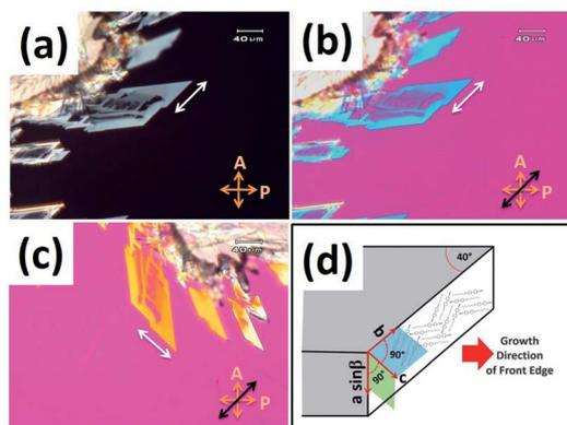
Fig. 2 The POM textures of a strip of PP phase between crossed polarisers: (a) without  $\lambda$ -plate, (b) with the slow axis of the  $\lambda$ -plate parallel to the front edge and (c) with the slow axis of the  $\lambda$ -plate perpendicular to the front edge. The white double headed arrow indicates the major axis of the effective refractive index ellipse within the strip. (d) The schematic representation of the molecular organisation within the strip.
