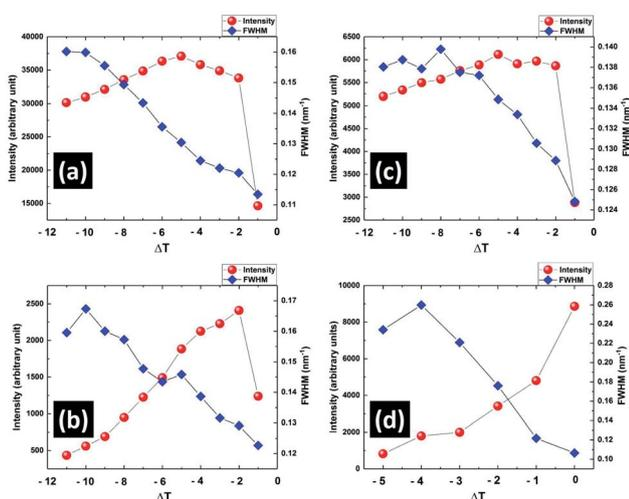
Fig. 7 The temperature variation of intensity and FWHM of three crystalline peaks (a) (100), (b) (001), (c) ( $10\bar{1}$ ) of CP phase and (d) (001) peak of smectic phase on heating the sample in the pre-transitional temperature range. Here  $\Delta T = T - T_c$ , where  $T$  and  $T_c$  denote the measured temperature and the complete melting temperature of CP phase respectively.
