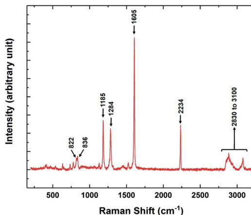
Fig. 9 The Raman spectrum of the stable CP phase of 8OCB showing the prominent vibrational peaks in the range from 200 cm<sup>-1</sup> to 3200 cm<sup>-1</sup>.
