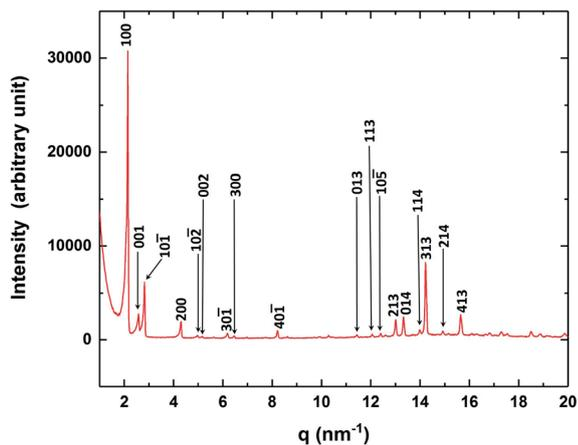
Fig. 6 The XRD intensity profile of the CP phase showing the characteristic peaks corresponding to a monoclinic lattice structure. The  $2\theta$  range corresponding to the  $q$ -range shown in the figure is from  $1^\circ$  to  $28^\circ$ . The Miller indices associated with the peaks are also depicted.
