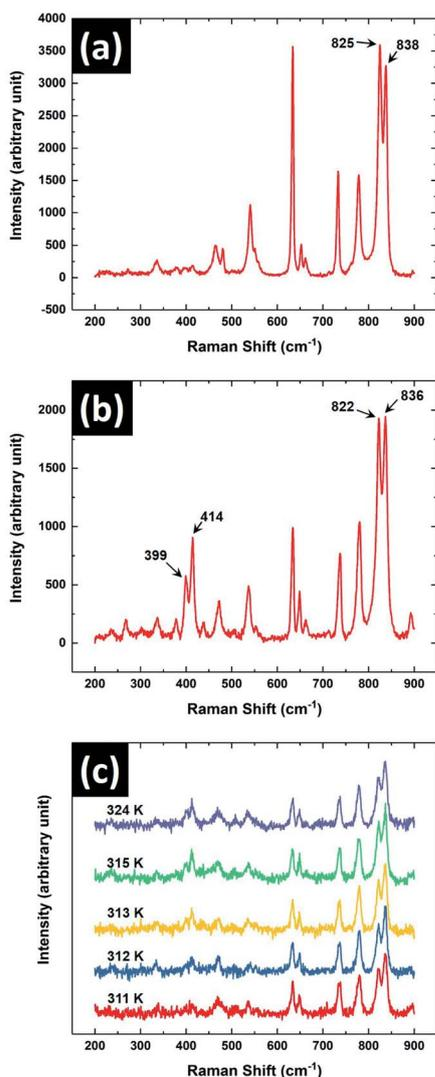
Fig. 8 The Raman spectrum in the range from 200 cm<sup>-1</sup> to 900 cm<sup>-1</sup> of 8OCB in its (a) PP phase and (b) CP phase. (c) The Raman spectra of 8OCB showing the variation with temperature across the transition from PP to CP phase.
