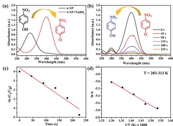
Fig. 7 UV-Vis spectra of (a) 4-NP before and after addition of  $\text{NaBH}_4$ , (b) time-dependent reduction process after the addition of Au/ATGO composites in the reaction. 4-NP reduction catalyzed by Au/ATGO composites in the presence of  $\text{NaBH}_4$ . (c) The plot of  $-\ln(C_t/C_0)$  versus time, and (d) the plot of  $\ln k$  versus  $1/T$  based at different temperatures.
