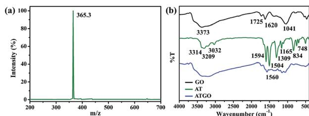
Fig. 1 (a) Mass spectra of AT. (b) FTIR spectra of GO, AT, and ATGO.
