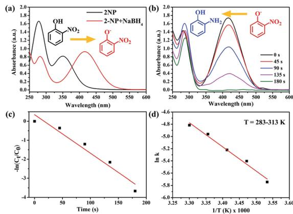
Fig. 8 UV-Vis spectra of (a) 2-NP before and after addition of  $\text{NaBH}_4$ , (b) time-dependent reduction process after the addition of Au/ATGO composites in the reaction. 2-NP reduction catalyzed by Au/ATGO composites in the presence of  $\text{NaBH}_4$ . (c) the plot of  $-\ln(C_t/C_0)$  versus time, and (d) the plot of  $\ln k$  versus  $1/T$  based on different temperature.
