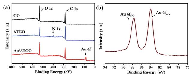
Fig. 3 XPS profiles of (a) GO, ATGO, and Au/ATGO; Au 4f spectra of (b) Au/ATGO composites.
