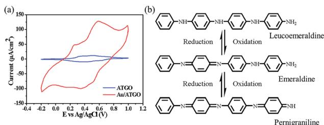
Fig. 6 Representative CV curves of the (a) ATGO and Au/ATGO composites in H<sub>2</sub>SO<sub>4</sub> solution. Scan rate: 50 mV s<sup>–1</sup>. (b) Molecular structures of ATGO at various oxidation states.
