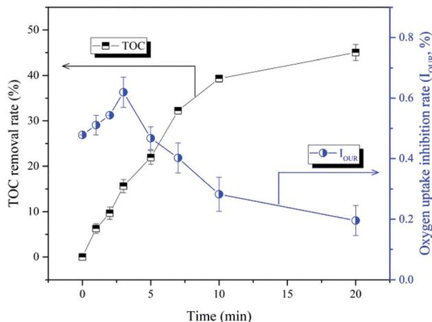
Fig. 13 Changes of TOC and bio-toxicity during BPA treatment in the nZVI/SPC system. Reaction conditions:  $[BPA]_0 = 0.1 \text{ mM}$ ,  $[nZVI]_0 = 0.1 \text{ g L}^{-1}$ ,  $[SPC]_0 = 3 \text{ mM}$ ,  $\text{pH}_0 = 4.0$ .
