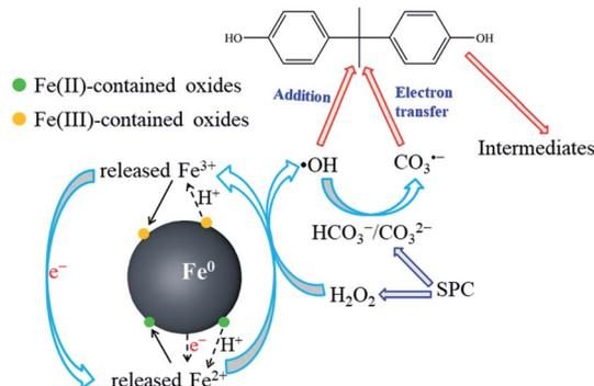
Fig. 11 Proposed mechanism of BPA degradation in the nZVI/SPC system.
