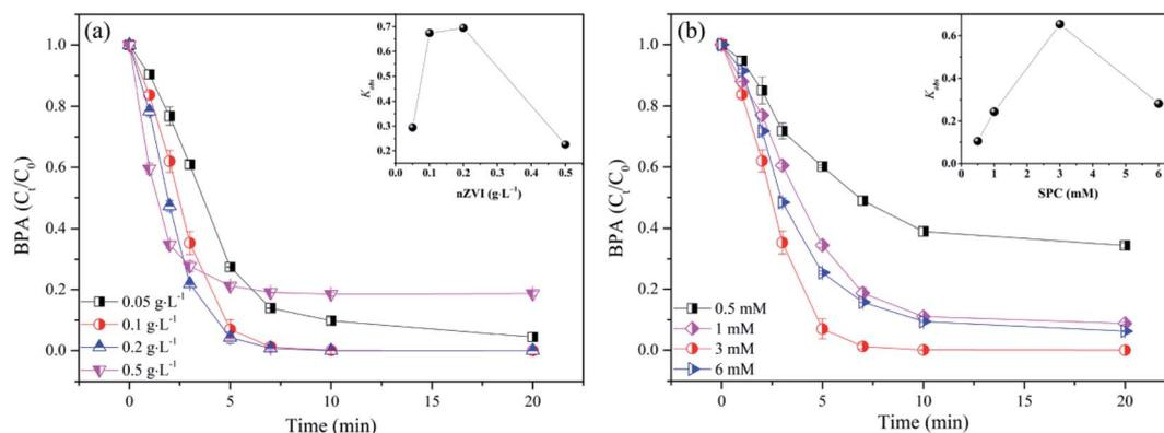
Fig. 4 Influence of nZVI loading (a) and SPC dosing (b) on BPA degradation in nZVI/SPC system: [BPA]<sub>0</sub> = 0.1 mM, [nZVI]<sub>0</sub> = 0.1 g L<sup>-1</sup>, [SPC]<sub>0</sub> = 3 mM, pH<sub>0</sub> = 4.0.
