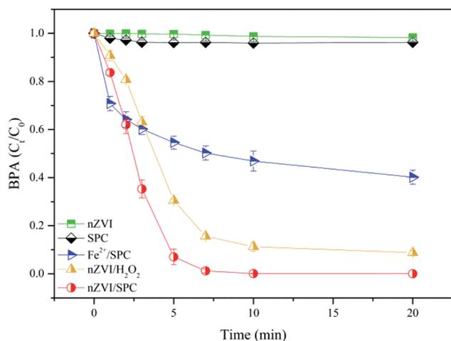
Fig. 1 BPA degradation in various systems. General reaction conditions:  $[\text{BPA}]_0 = 0.1 \text{ mM}$ ,  $[\text{nZVI}]_0 = 0.1 \text{ g L}^{-1}$ ,  $[\text{Fe}^{2+}]_0 = 2.3 \text{ mg L}^{-1}$ ,  $[\text{H}_2\text{O}_2]_0 = 4.5 \text{ mM}$ ,  $[\text{SPC}]_0 = 3 \text{ mM}$ ,  $\text{pH}_0 = 4.0$ .
