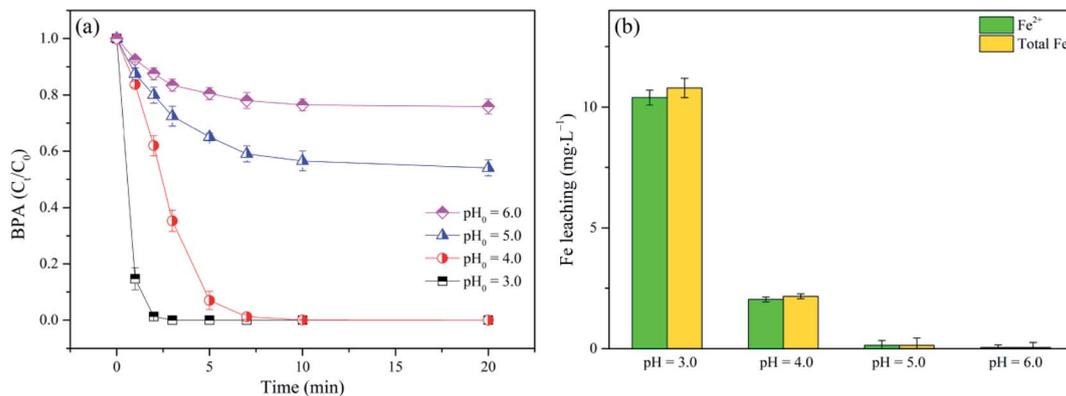
Fig. 5 (a) Effect of  $\text{pH}_0$  on BPA degradation; (b) Fe leaching in the nZVI/SPC system. General reaction conditions:  $[\text{BPA}]_0 = 0.1 \text{ mM}$ ,  $[\text{nZVI}]_0 = 0.1 \text{ g L}^{-1}$ ,  $[\text{SPC}]_0 = 3 \text{ mM}$ .
