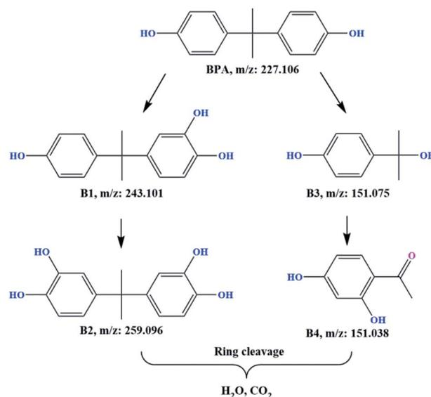
Fig. 12 Possible degradation pathway of BPA in the nZVI/SPC system. Reaction conditions: [BPA]<sub>0</sub> = 0.1 mM, [nZVI]<sub>0</sub> = 0.1 g L<sup>-1</sup>, [SPC]<sub>0</sub> = 3 mM, pH<sub>0</sub> = 4.0.
