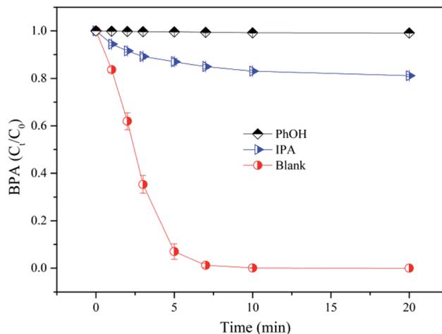
Fig. 8 The effects of IPA and PhOH on BPA degradation in nZVI/SPC system. General reaction conditions:  $[BPA]_0 = 0.1$  mM,  $[nZVI]_0 = 0.1$  g L<sup>-1</sup>,  $[SPC]_0 = 3$  mM,  $pH_0 = 4.0$ .
