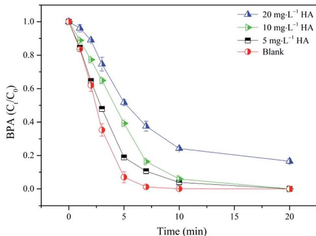
Fig. 7 Effect of HA on BPA degradation in the nZVI/SPC system:  $[BPA]_0 = 0.1$  mM,  $[nZVI]_0 = 0.1$  g L<sup>-1</sup>,  $[SPC]_0 = 3$  mM,  $pH_0 = 4.0$ .
