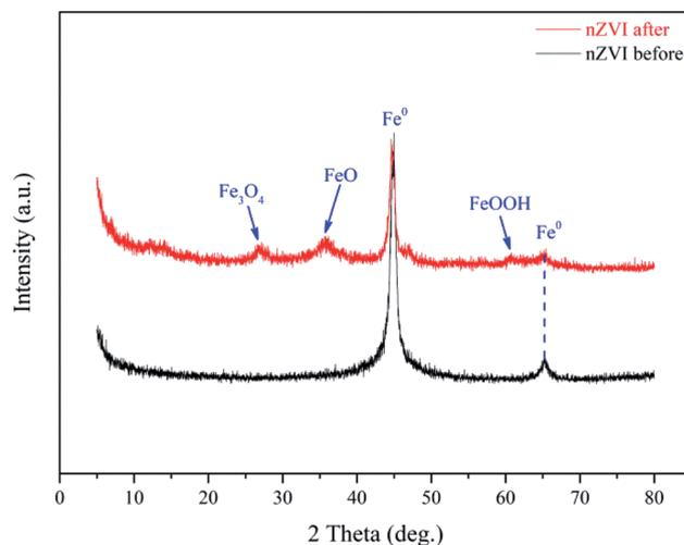
Fig. 9 XRD of nZVI before and after use.
