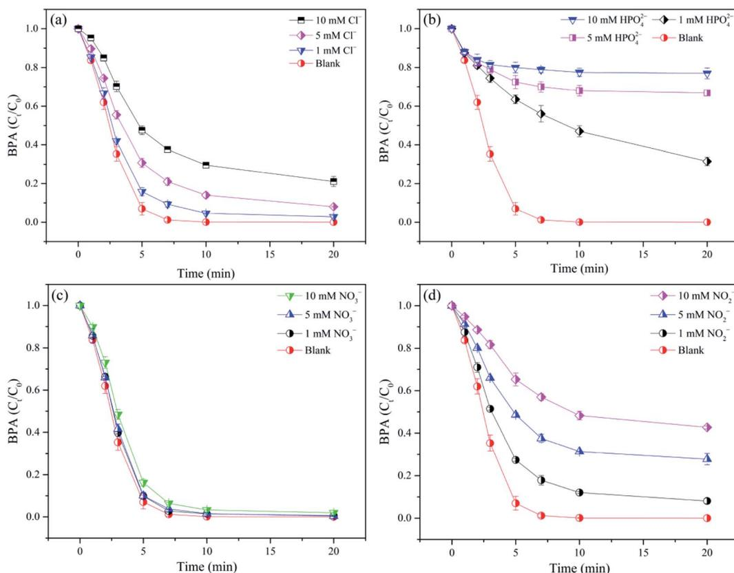
Fig. 6 Effect of anions on BPA degradation in nZVI/SPC system. (a)  $\text{Cl}^-$ ; (b)  $\text{HPO}_4^{2-}$ ; (c)  $\text{NO}_3^-$ ; (d)  $\text{NO}_2^-$ . React conditions:  $[\text{BPA}]_0 = 0.1 \text{ mM}$ ,  $[\text{nZVI}]_0 = 0.1 \text{ g L}^{-1}$ ,  $[\text{SPC}]_0 = 3 \text{ mM}$ ,  $\text{pH}_0 = 4.0$ .
