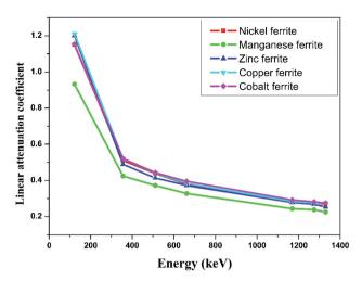
Fig. 3 Experimental linear attenuation coefficients ( $\mu$ ) *versus* incident photon energy.
