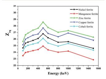
Fig. 10 Experimental study of equivalence atomic number ( $Z_{\rm eq}$ ) against incident photon energy.
