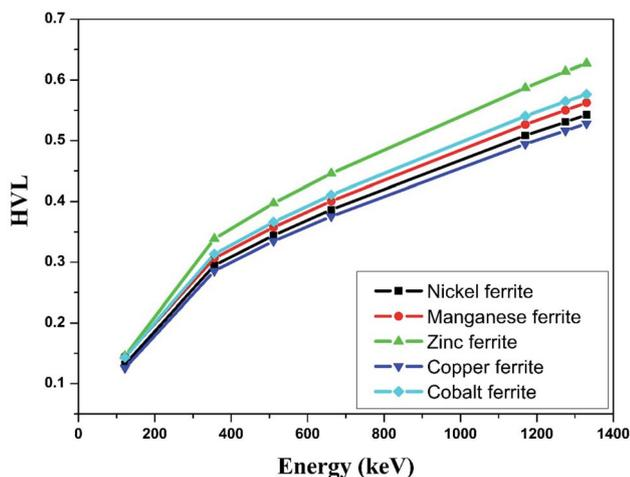
Fig. 9 Experimental study of half value layer against incident photon energy.
