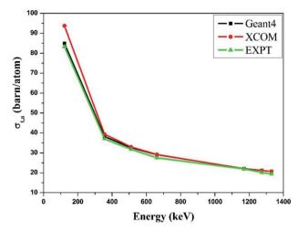
Fig. 5 Comparative study of the total atomic cross-section ( $\sigma_{t,a}$ ) verses incident photon energy for zinc ferrite.
