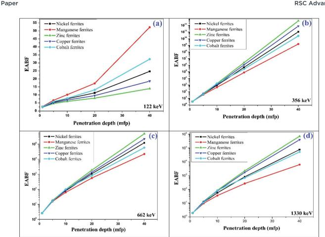
Fig. 12 Typical plot of penetration depth against EABF at (a) 122 keV, (b) 356 keV, (c) 662 keV and (d) 1330 keV photon energy for the synthesized
