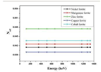
Fig. 8 Experimental study of effective electron density ( $N_{\rm eff}$ ) against incident photon energy.
