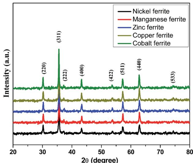
Fig. 1 X-ray diffractograms for the produced spinel nano-ferrites.
