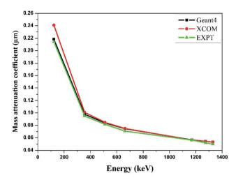
Fig. 4 Comparison of experimental and theoretical mass attenuation coefficient against incident photon energy for zinc ferrite.
