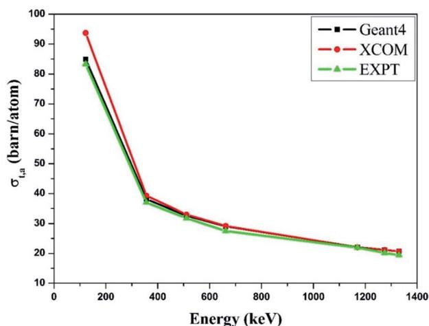
Fig. 5 Comparative study of the total atomic cross-section ( $\sigma_{t,a}$ ) versus incident photon energy for zinc ferrite.
