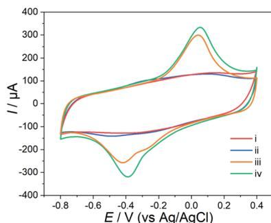
Fig. 3 CVs obtained at different modified electrodes in  $0.10$  M PBS at a scan rate of  $100$   $\text{mV s}^{-1}$ . (i) rGO/GCE, (ii) Hemin/rGO/GCE, (iii) HKUST-1/rGO/GCE and (iv) Hemin-doped-HKUST-1/rGO/GCE.
