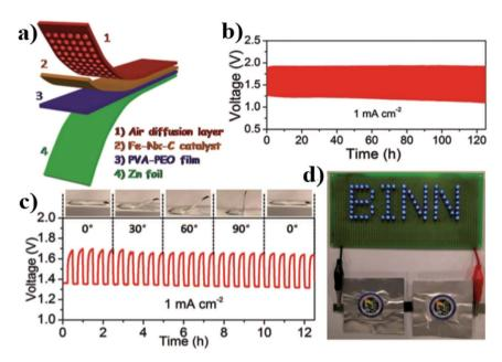
Fig. 12 (a) Schematic of all-solid-state ZAB. (b) Cycling performance of the all-solid-state ZAB tested at a current density of 1 mA cm $^{-2}$ . (c) Foldability test of all-solid-state ZAB bended in different angles from 0° to 90° at a current density of 1 mA cm $^{-2}$ . (d) A lighted LED array powered by two all-solid-state ZABs in series.
