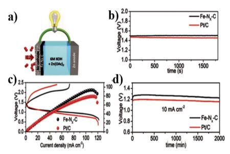
Fig. 11 (a) Schematic showing the structure of ZAB. (b) OCV plots of the liquid ZABs. (c) Discharging and charging polarization curves and the corresponding power density plots. (d) Long-term discharging performance of primary ZABs.
