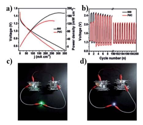
Fig. 14 (a) Discharge polarization curves and the corresponding power density curves of primary zinc-air batteries using the N-FC-800 as air catalysts (mass loading of 1 mg cm $^{-2}$ ); (b) cycling performance of rechargeable zinc-air batteries at a current density of 10 mA cm $^{-2}$ ; (c and d) photographic images of a two-electrode rechargeable zinc-air battery lighting up a LED light (blue for (c) and white for (d)).
