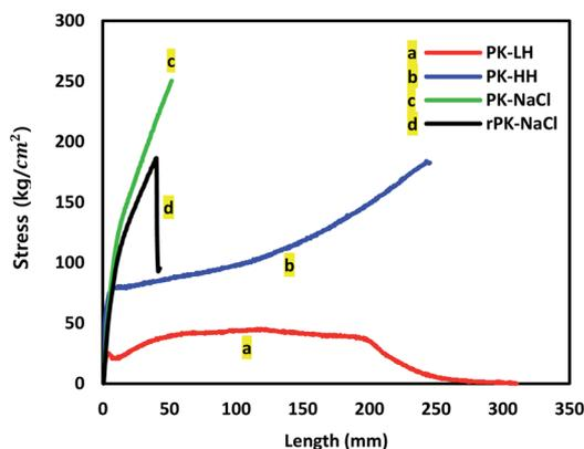
**Fig. 6** Tensile strength of PK micro/nano fiber membranes.
