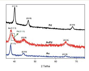
Fig. 2 XRD pattern of Pd, Au and AuPd
