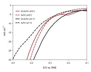
Fig. 5 LSV polarization curves of AuPd and EA-AuPd electrocatalyst for the HER. Measurements were conducted in 0.5 M  $H_2SO_4$  (pH 0.3) and in 1 M NaOH (pH 14) at a scan rate of 50 mV s<sup>-1</sup>.
