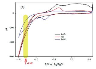
Fig. 4 (a) Chronoamperograms of AuPd, Pd and Pd/C at -1.3 V in PBS (pH 8.4), (b) cyclic voltammograms (CV) of AuPd, Pd and Pd/C in PBS (pH 8.4), scan rate: 50 mV s $^{-1}$ .
