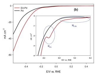
Fig. 3 LSV polarization curves for HER on: (a) AuPd and EA-AuPd electrocatalysts, (b) Pd and EA-Pd electrocatalysts. The insets show zoom-in at lower current density. Measurements were conducted in 1 M NaOH solutions at a scan rate of 50 mV s $^{-1}$ .
