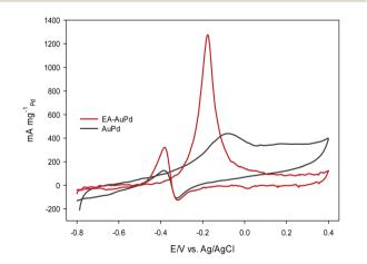
Fig. 6 CV curves of AuPd and EA-AuPd in 1 M NaOH + 1 M methanol at a scan rate of 50 mV s $^{-1}$ .
