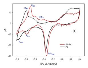
Fig. 9 Comparison of CV curves in 1.0 M NaOH solution for the (a) AuPd and (b) Pd, before and after being subjected to EA process (scan rate 50 mV s $^{-1}$ ).
