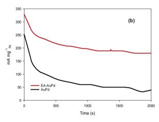
Fig. 8 (a) Dependence of anodic current peak for EA-AuPd and AuPd catalysts on cycle number. (b) Chronoamperometry curves of EA-AuPd and AuPd catalysts for the MOR measured at -0.18 V (vs. Ag/AgCl). All experiments were conducted in 1 M methanol + 1 M NaOH.
