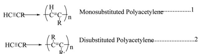
Scheme 1 Formation of monosubstituted and disubstituted polyacetylene.
