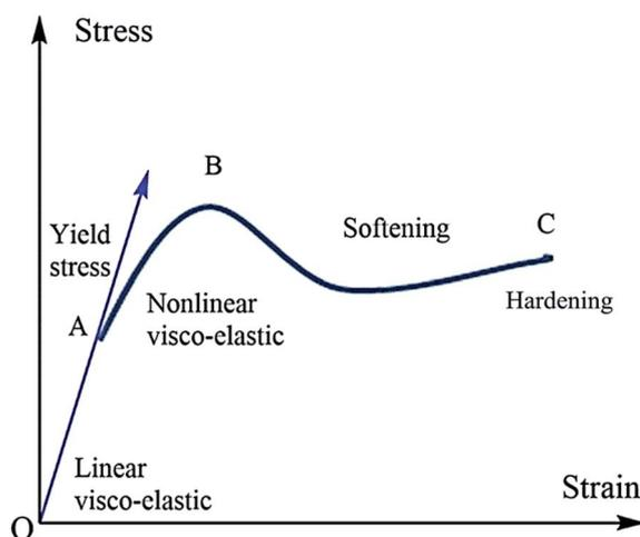
Fig. 8 Typical stress–strain curve of polymeric materials.
