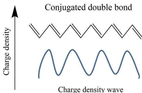
Fig. 6 Representation of charge density wave in polyacetylene.
