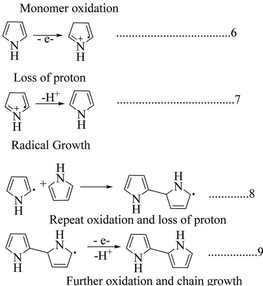
Scheme 5 Mechanism of electrochemical synthesis of polypyrrole.
