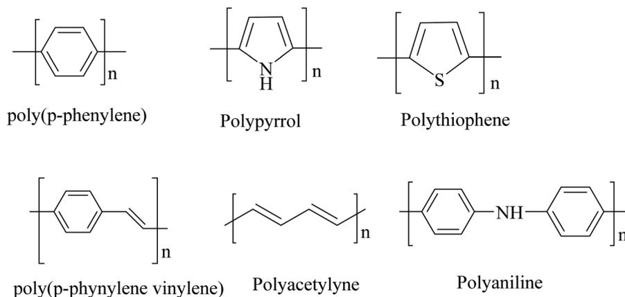
Chart 1 Structural illustration of different conducting polymers.
