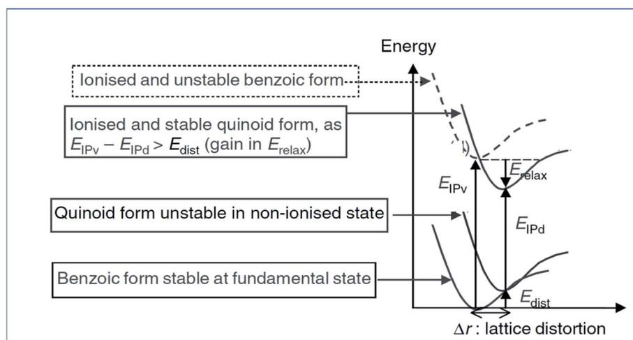
Fig. 5 Energy level diagram of the molecular ionization process of poly(*p*-phenylene) (reprinted with permission,<sup>65</sup> copyright 2004 Wiley).
