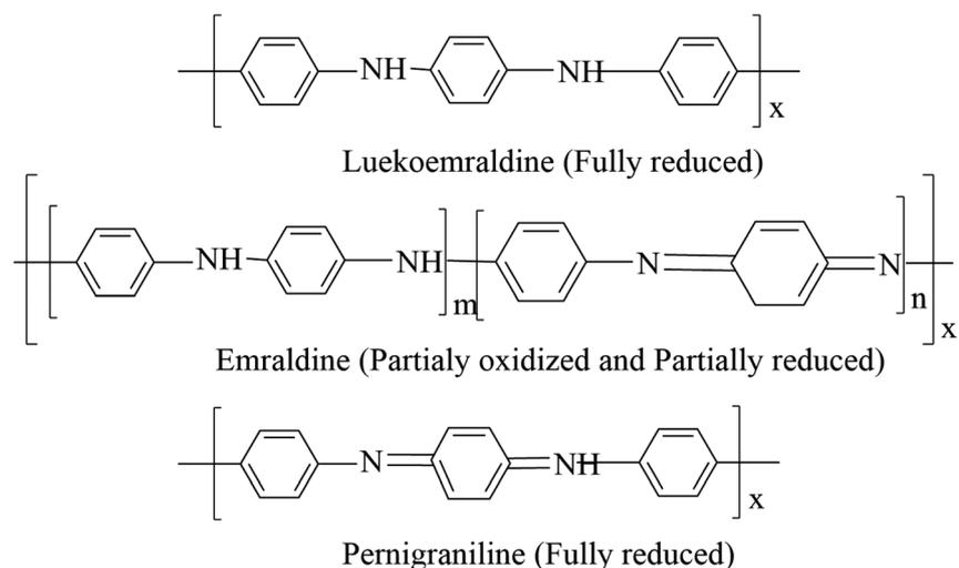
Chart 2 Structural illustration of different forms of polyaniline.
