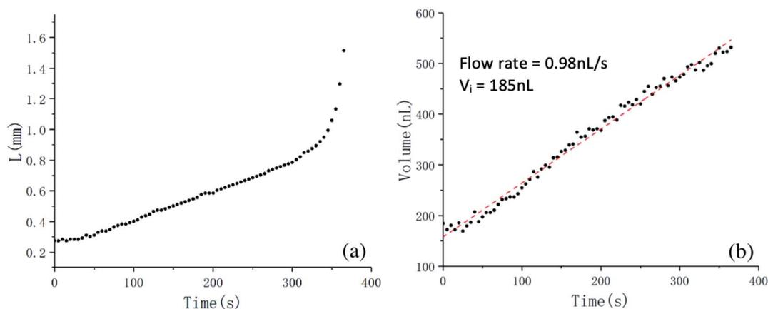
Fig. 3 (a) Meniscus length in the axial direction as a function of time. (b) Volume of PCL melt at the nozzle *versus* time. A 2.7 kV high voltage is applied to the nozzle when the volume of PCL melt is 185 nL. The flow rate is  $0.98 \text{ nL s}^{-1}$ , estimated from the linear fitting.
