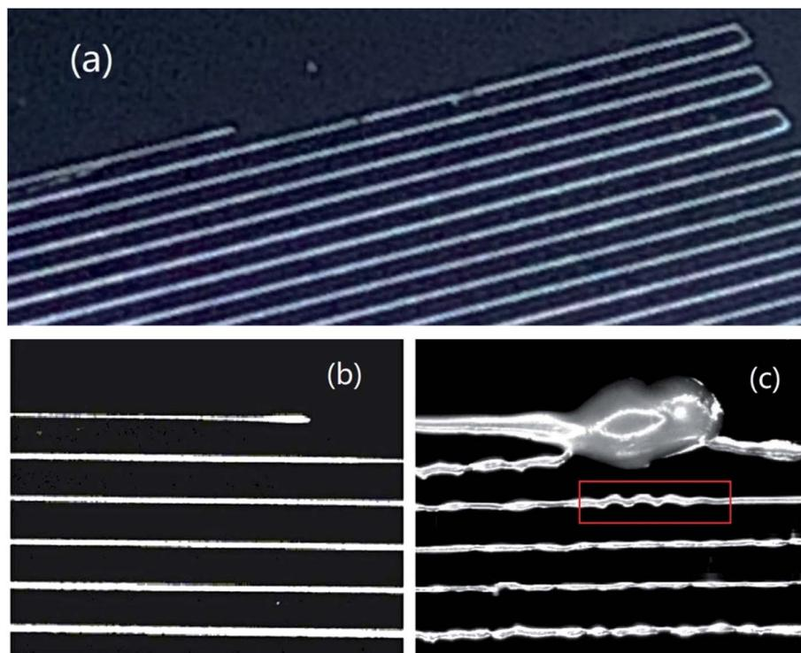
Fig. 8 The printing of a meander pattern. The printing begins as long as the liquid touches the substrate, with plotting speed of  $0.6 \text{ mm s}^{-1}$ . For (a) and (b), nozzle voltage is applied when the PCL melt volume  $V_i$  is 182 nL. For (c),  $V_i$  is 514 nL.
