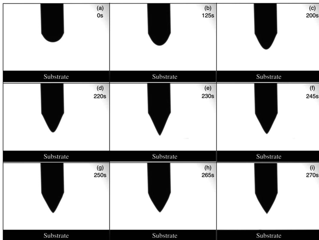
Fig. 6 The process of meniscus deformation. A 2.7 kV high voltage is applied to the nozzle when the volume of PCL melt is 360 nL.
