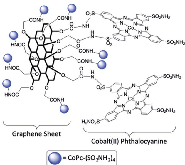
Fig. 22 Graphene-tethered cobalt(II) phthalocyanine catalyst for heterogeneous photoconversion of CO<sub>2</sub> to methanol.<sup>174</sup>
