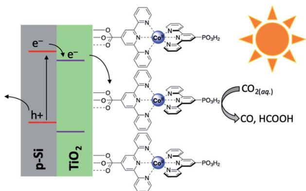
Fig. 10 Schematic diagram of p-Si/meso- $\text{TiO}_2$ /CotpyP photocathode used in photoelectrolytic reduction of  $\text{CO}_2$ .<sup>107</sup>
