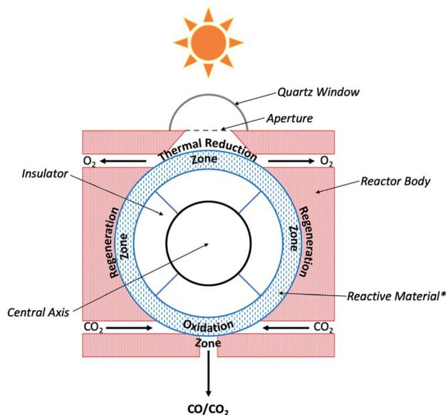
Fig. 8 Schematic diagram of CR5 used for  $\text{CO}_2$  photoconversion. \*Reactive material is comprised of sets of counter-rotating rings. Current cross-sectional view shows single ring oriented coincident with the plane of this page.<sup>83,84</sup>
