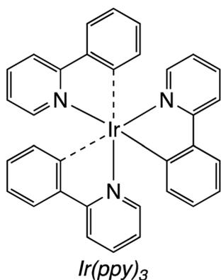
Fig. 18 Iridium photosensitiser (Ir(ppy)<sub>3</sub>) studied in the FeCAT-mediated photoconversion of carbon dioxide to carbon monoxide.<sup>158</sup>
