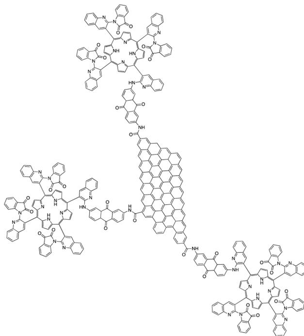
Fig. 24 CCG-IP photocatalyst used in photocatalytic/biocatalytic reduction of CO<sub>2</sub> to methanol.<sup>183</sup>
