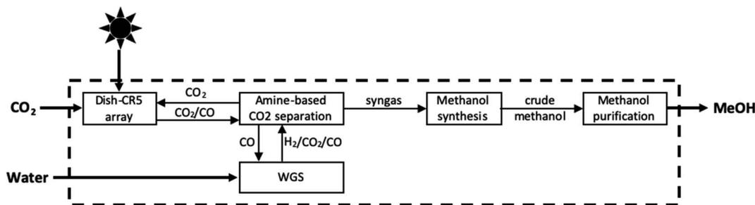
Fig. 9 Block flow diagram of photothermal conversion of CO<sub>2</sub> to methanol by S2P process.<sup>84</sup>
