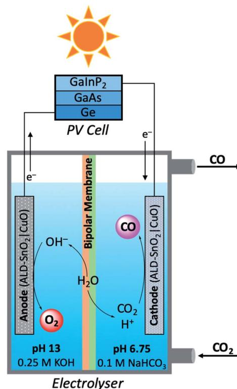
Fig. 11 Schematic diagram of modular photoelectrolyser used in carbon dioxide reduction mediated by bifunctional ALD- $\text{SnO}_2$ /CuO electrodes.<sup>109</sup>
