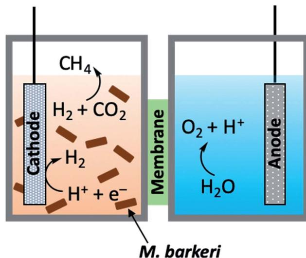
Fig. 13 General schematic diagram of hybrid bio-PEC cell.<sup>118</sup>
