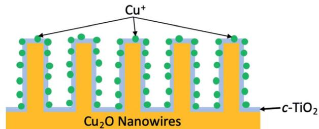
Fig. 12 Schematic cross-sectional view of Cu<sub>2</sub>O|TiO<sub>2</sub>-Cu<sup>+</sup> photocathode.
