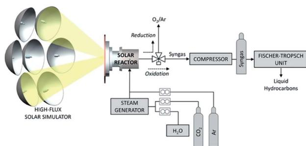
Fig. 7 Schematic diagram of solar reactor used in the ceria-mediated photothermal reduction of carbon dioxide. Image adapted with permission from ACS Publications.<sup>79</sup>
