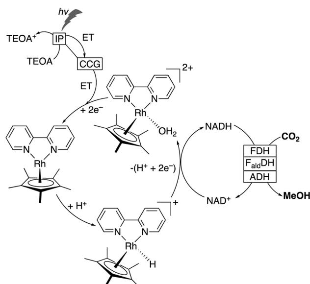
Fig. 25 Proposed mechanism of photocatalytic/biocatalytic conversion of carbon dioxide to methanol.<sup>183</sup>
