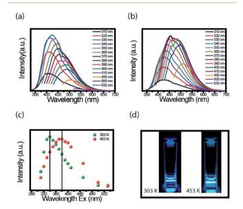
Fig. 4 Excitation-dependent PL emission spectra. (a) Heating 303 K and (b) heating 453 K. (c) The wavelength of highest intensity from emission-dependent PL at 303 K, plot (a), (green dots) and 453 K, plot (b), (red dots). (d) The photographs of fluorescent CDs under laser excitation 380 nm.
