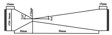
Fig. 3 Venturi tube size.
