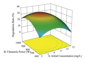
Fig. 4 The effect of the interaction between ultrasonic power and initial concentration on degradation. (a) Respond the surface cloud chart; (b) contour map.
