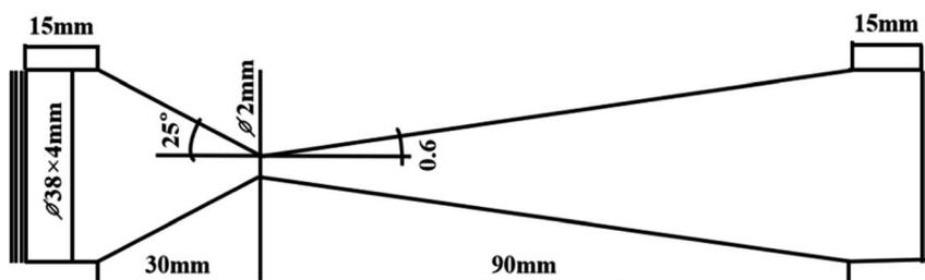
Fig. 3 Venturi tube size.
