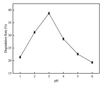
Fig. 9 The effect of pH on degradation rate with hydrodynamic cavitation.
