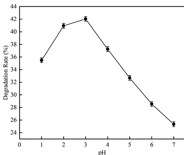
Fig. 7 The effect of pH on degradation rate with ultrasonic cavitation.
