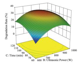
Fig. 6 The effect of the interaction of ultrasound time and ultrasound power on degradation rate. (a) Respond the surface cloud chart; (b) contour map.
