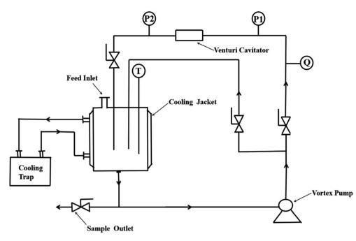
Fig. 2 Hydraulic cavitation device.
