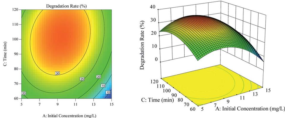
Fig. 5 The effect of the interaction of ultrasound time and initial concentration on degradation rate. (a) Respond the surface cloud chart; (b) contour map.
