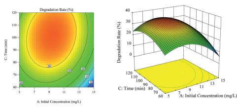
Fig. 5 The effect of the interaction of ultrasound time and initial concentration on degradation rate. (a) Respond the surface cloud chart; (b) contour map.
