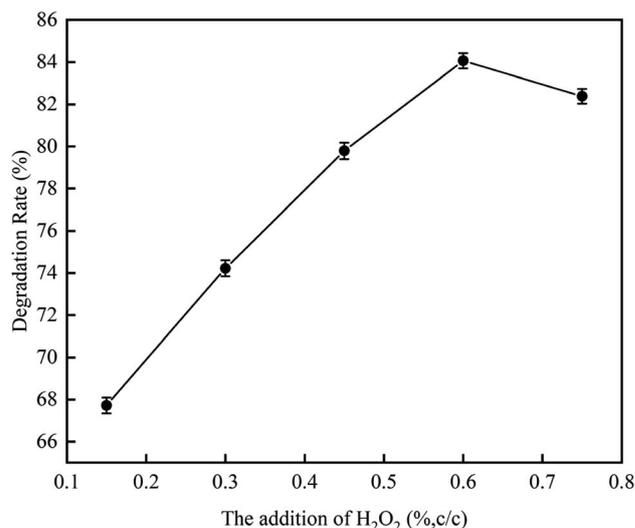
Fig. 8 The effect of H<sub>2</sub>O<sub>2</sub> addition on degradation rate with ultrasonic cavitation.
