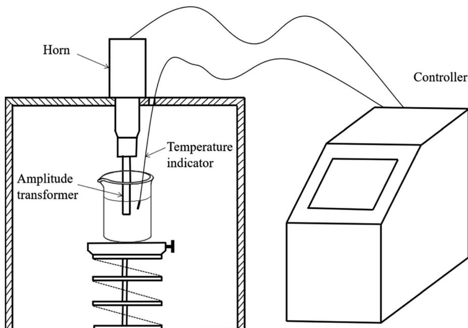
Fig. 1 Schematic diagram of ultrasonic cavitation device.
