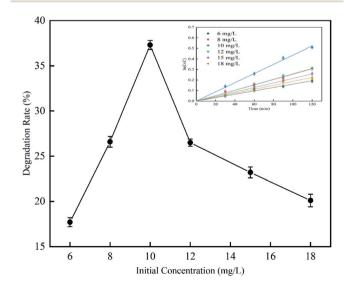
Fig. 11 The effect of initial concentration on degradation rate with hydrodynamic cavitation.
