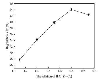
Fig. 8 The effect of H<sub>2</sub>O<sub>2</sub> addition on degradation rate with ultrasonic cavitation.
