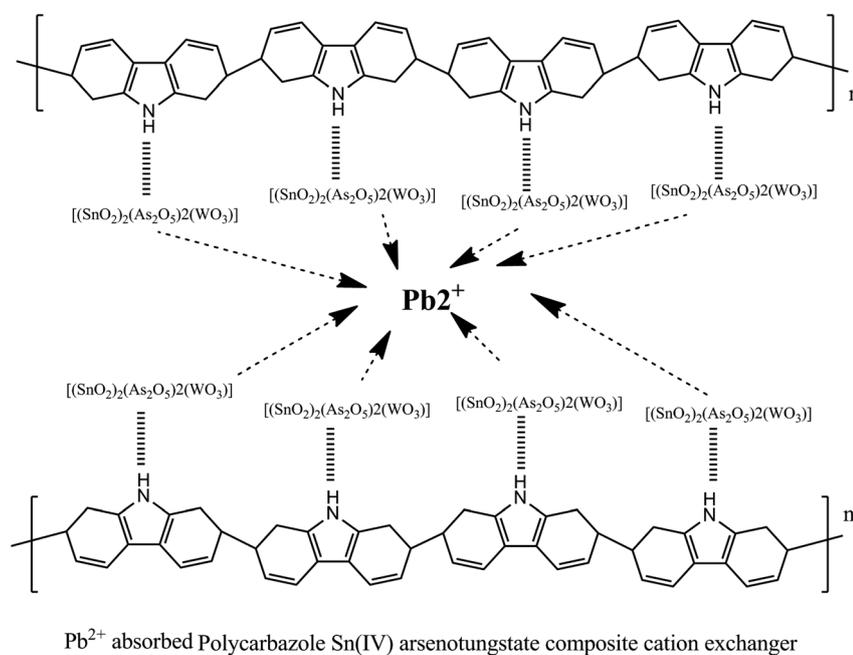
Schematic interaction of  $\text{Pb}^{2+}$  with Polycarbazole Sn(IV) arsenotungstate composite cation exchangerScheme 2 The schematic of the formation of Pcz-SnAT IEM interactions with  $\text{Pb}^{2+}$ .
