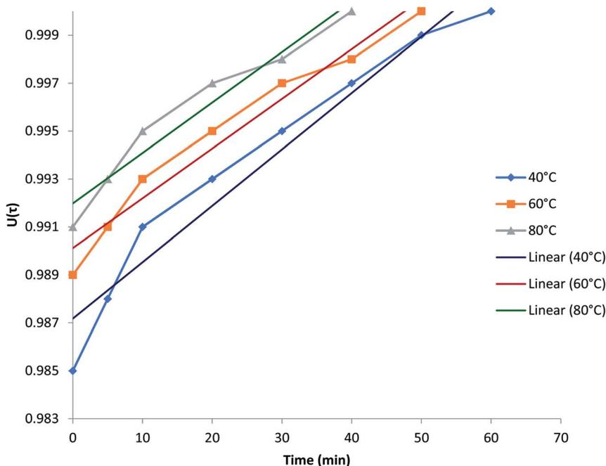
Fig. 6 Plots of  $U(\tau)$  versus  $t$  (time) for Pb(II)-H<sup>+</sup> exchanges at different temperatures: 40 °C, 60 °C and 80 °C of the Pcz-SnAT composite IEM electrode.
