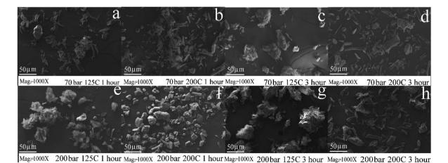
Fig. 8 SEM images of cellulose after the hydrothermal process at 1000× magnification, at a pressure of 70 bar; after the hydrothermal process for 1 hour at (a) 125 °C and (b) 200 °C; after the hydrothermal process for 3 hours at (c) 125 °C and (d) 200 °C. At a pressure of 200 bar; after the hydrothermal process for 1 hour at (e) 125 °C and (f) 200 °C; after the hydrothermal process for 3 hours at (q) 125 °C and (h) 200 °C.
