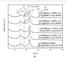
Fig. 5 Variation in the XRD patterns of the effects of hydrothermal processing at  $CO_2$  pressures of 70 bar (a) and 200 bar (b); for each temperature of 125 °C and 200 °C, for various times of degradation.
