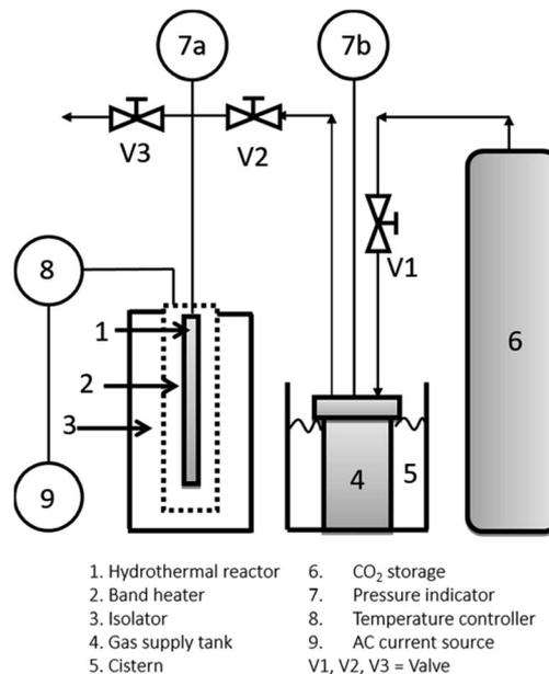
Fig. 2 Experimental apparatus for the hydrothermal process.
