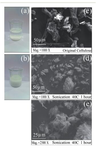
Fig. 3 Mixture of cellulose in a solution of oxalic acid  $(H_2C_2O_4)$ –sodium chloride (NaCl), (a) without sonication, (b) after sonication. (c) SEM photograph of cellulose without sonication, and (d) and (e) after sonication.
