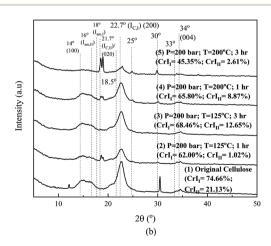
Fig. 9 Variation in the XRD patterns of the effects of ultrasonic pretreatment followed by hydrothermal processing at  $CO_2$  pressures of 70 bar (a) and 200 bar (b); for each temperature of 125 °C and 200 °C, for various times of degradation.
