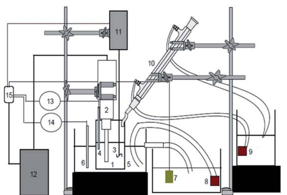
Fig. 1 Experimental apparatus for the sonication process.
