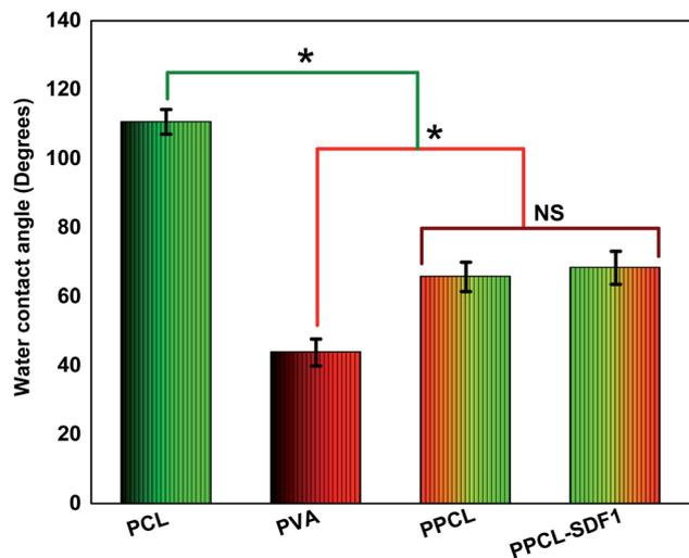
Fig. 4 The water contact angles of PCL, PVA, PPCS, and PPCS-SDF1 membranes. (\*) indicates  $p$ -values where a statistically significant difference ( $p \leq 0.05$ ) is observed. NS indicates no statistically significant difference.
