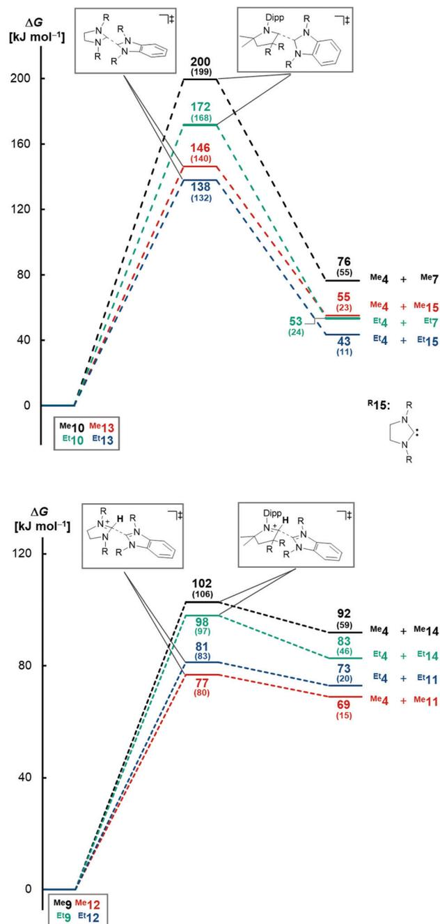
**Fig. 1** Calculations at the DLPNO-CCSD(T)/def2-TZVPP//BLYP-D3BJ/def2-TZVPP level of theory quantify acid catalysis for dissociation of tri- and tetraaminoolefins. Values in parentheses relate to implicit solvation in THF.
