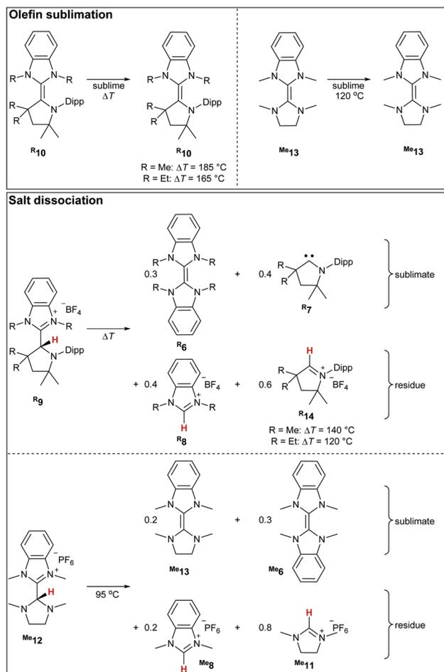
**Scheme 4** Whereas sublimation was observed for the electron-rich olefins **R10** and **Me13** (top), dissociation and subsequent separation of volatile and non-volatile products were obtained for their protonated congeners **R9** and **Me12** (bottom). All experiments were conducted at  $5 \times 10^{-3}$  mbar.
