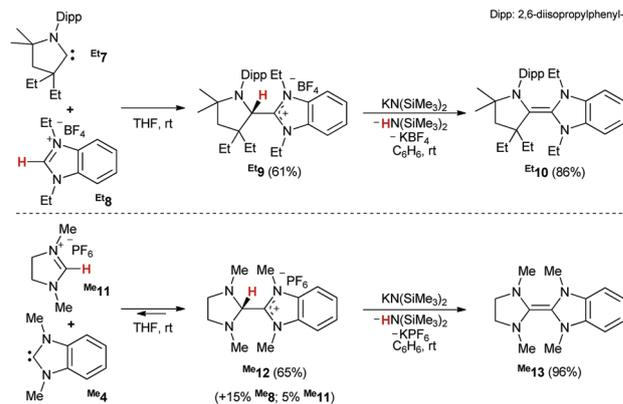
**Scheme 3** The CAAC-derived protonated heterodimer **Et9** and olefins **Et10**, **Me13** do not dissociate in solution at room temperature (top), whereas saNHC-derived **Me12** stands in equilibrium with the starting materials **Me4** and **Me11**.
