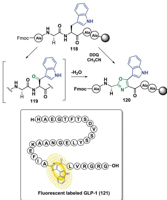
**Scheme 31** Site-selective formation of oxazole-based fluorophores by Qvortrup *et al.*<sup>102</sup>
