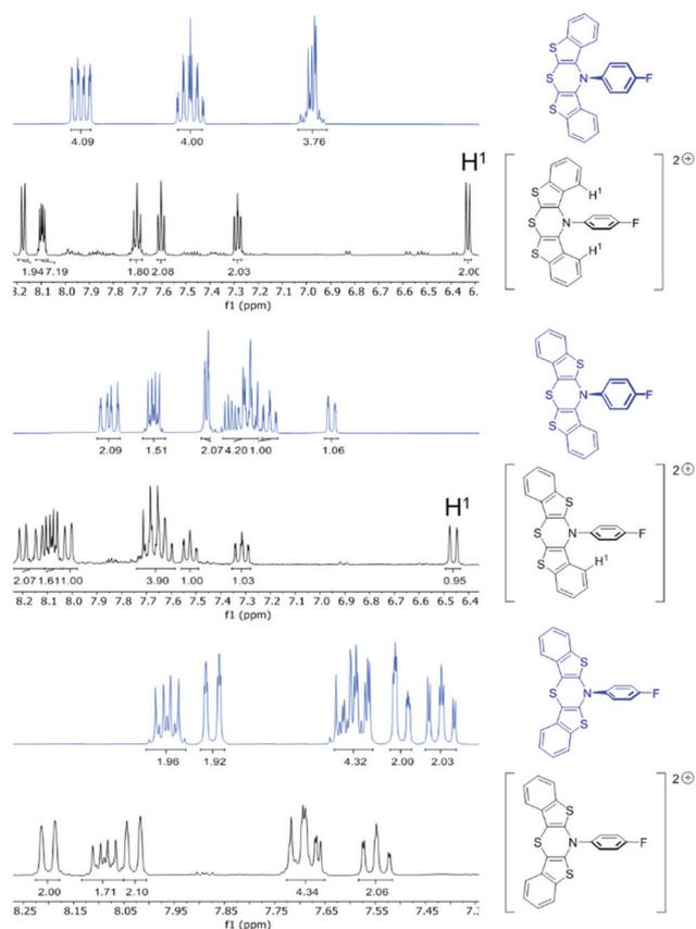
**Fig. 4** Sections of the  $^1\text{H}$  NMR spectra of the neutral compounds **5**, **6**, and **7** (blue) and of the bis(hexachloro-antimonate) salts of  $5^{2+}$ ,  $6^{2+}$ , and  $7^{2+}$  (black) (300 MHz, acetone- $d_6$ ,  $T = 298$  K).
