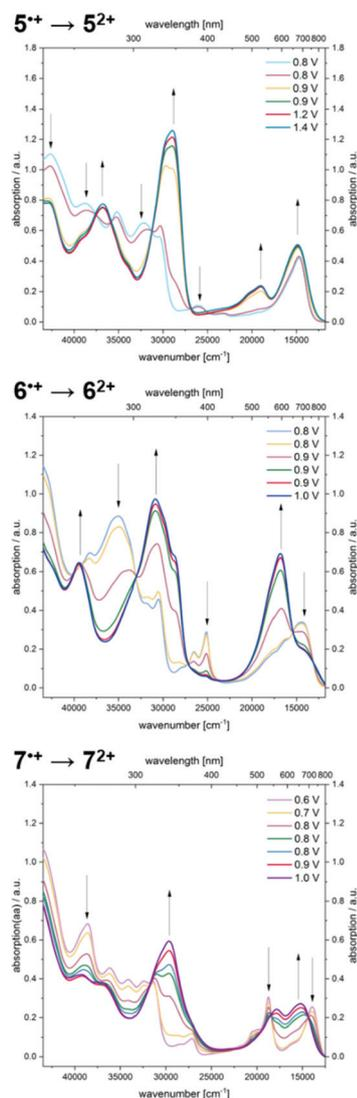
**Fig. 8** UV/Vis spectroelectrochemical measurements of radical cations  $5^+$ ,  $6^+$ , and  $7^+$  forming the corresponding dicationic species  $5^{2+}$ ,  $6^{2+}$ , and  $7^{2+}$  ( $\text{CH}_2\text{Cl}_2$ ,  $T = 293$  K; electrolyte 0.1 M  $[\text{tBu}_4\text{N}][\text{PF}_6]$ ; Pt working electrode, Pt counter electrode and Ag/AgCl pseudo reference electrode).
