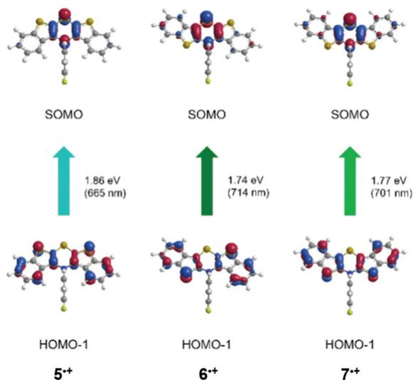
**Fig. 11** TDDFT calculated molecular orbital transitions of most bathochromic absorptions of radical cations 5<sup>+</sup>, 6<sup>+</sup>, and 7<sup>+</sup> (uB3LYP/6-311++G\*\*, IEFPCM CH<sub>2</sub>Cl<sub>2</sub>, isosurface value 0.05 a.u.) (For further molecular orbital transitions, see SI).
