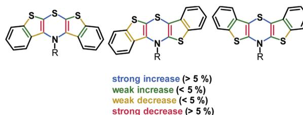
Fig. 3 Relative change of Wiberg bond orders  $\Delta(\text{BO}_{x+}-\text{BO}_x)$  from neutral precursors 5, 6, and 7 to radical cations 5<sup>•+</sup>, 6<sup>•+</sup>, and 7<sup>•+</sup> in the BBTT core (R = *p*-fluorophenyl; uB3LYP/6-311G\*\*) (A detailed list of bond orders is given in the ESI†).
