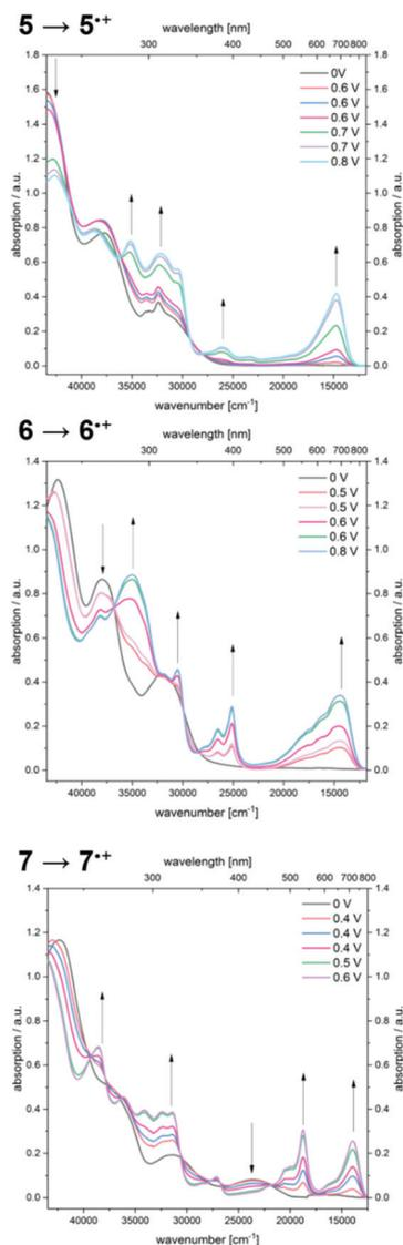
**Fig. 7** UV/Vis spectroelectrochemical measurements of compounds **5**, **6**, and **7** forming the corresponding radical cations  $5^+$ ,  $6^+$ , and  $7^+$  ( $\text{CH}_2\text{Cl}_2$ ,  $T = 293$  K; electrolyte 0.1 M  $[\text{tBu}_4\text{N}][\text{PF}_6]$ ; Pt working electrode, Pt counter electrode and Ag/AgCl pseudo reference electrode).
