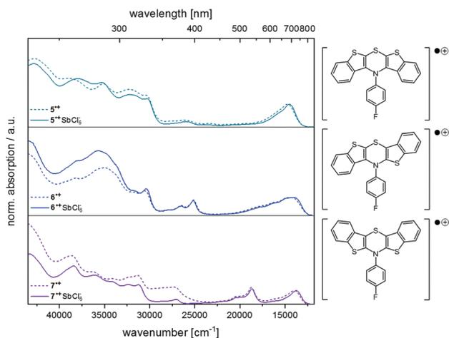
**Fig. 9** Comparison of the UV/Vis spectra from measurements of the radical cation salts (solid lines) and from spectroelectrochemical measurements (dotted lines) ( $\text{CH}_2\text{Cl}_2$ ,  $T = 293 \text{ K}$ , for further details, see ESI†).
