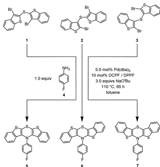
**Scheme 2** Selective synthesis of regioisomeric *N-p*-fluorophenyl-BBTTs **5**, **6**, and **7** prepared by cyclizing Buchwald–Hartwig amination (for the synthesis of compounds **5** and **6** DCPF (1,1'-bis(dicyclohexylphosphano)ferrocene) was employed as a ligand, and for compound **7** DPPF (1,1'-bis(diphenylphosphano)ferrocene) was used as a ligand).<sup>28</sup>
