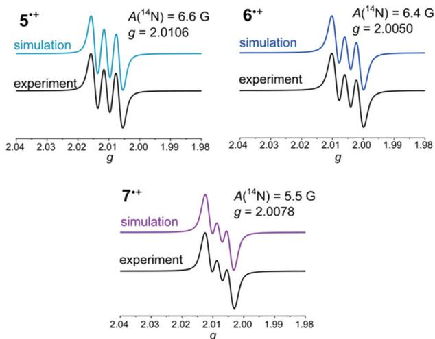
Fig. 2 Simulated and experimental EPR spectra of hexachloroantimonate salts of 5<sup>•+</sup>, 6<sup>•+</sup>, and 7<sup>•+</sup> (recorded in THF, *T* = 298 K, *g*-factor referenced to external Mn<sup>2+</sup> in ZnS).
