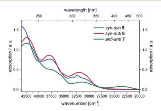
Fig. 5 UV/Vis spectra of compounds 5, 6, and 7 in the spectroelectrochemical cell at zero potential ( $CH_2Cl_2$ , T = 293 K).
