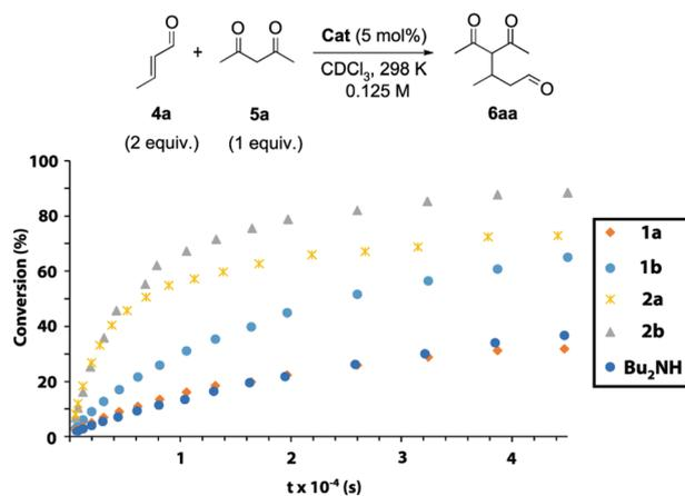
**Fig. 4** Plot of the conversion (%) *versus* time of the Michael addition between crotonaldehyde and acetylacetone catalyzed by: thread **1a** ( $\blacklozenge$ ), thread **1b** ( $\bullet$ ), rotaxane **2a** ( $\times$ ), rotaxane **2b** ( $\blacktriangle$ ) and dibutylamine ( $\bullet$ ). The conversion was determined by  $^1\text{H}$  NMR using  $\text{CH}_2\text{Br}_2$  as an internal standard.
