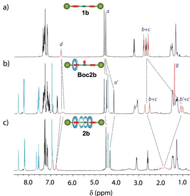
**Fig. 3** Stacked  $^1\text{H}$  NMR spectra (400 MHz,  $\text{CDCl}_3$ , 298 K) of (a) thread **1b**; (b) compartmentalised [2]rotaxane **Boc2b**; and (c) degenerate [2]rotaxane **2b**. See lettering in Figure 2.
