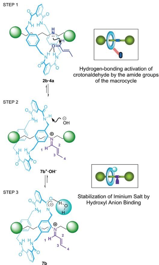
**Fig. 7** Proposed pathways for the formation of iminium intermediate **7b**: (step 1) hydrogen-bonding activation of crotonaldehyde **4a**; (step 2) formation of iminium salt **7b<sup>+</sup>·OH<sup>-</sup>**; (step 3) macrocycle-assisted hydroxyl anion binding for the stabilization of zwitterion **7b**.
