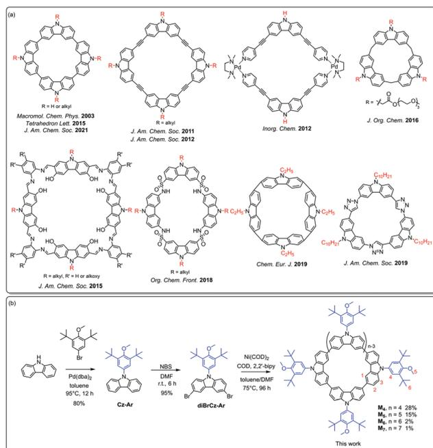
**Scheme 1** (a) Chemical structures of some representative carbazole-based macrocycles in the literature. (b) Synthesis of the macrocycles  $M_n$  ( $n = 4-7$ ) consisting of *N*-(3,5-di-*tert*-butyl-4-methoxyphenyl) substituted carbazole (Cz-Ar).
