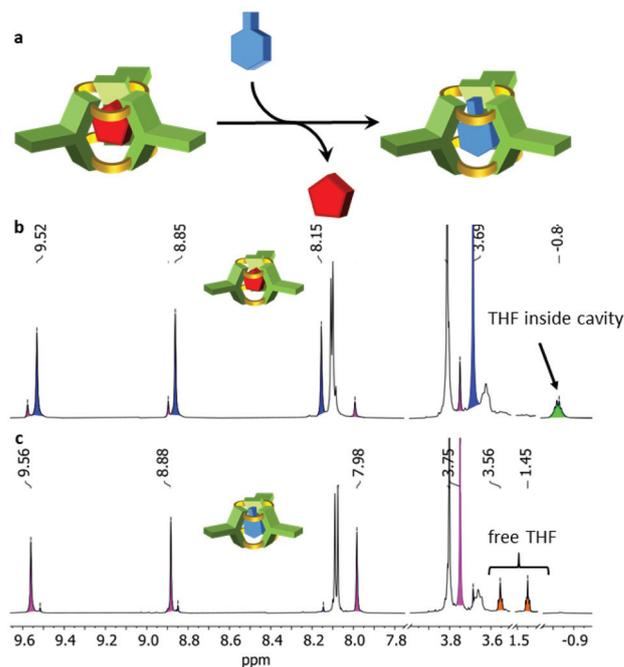
**Fig. 6** (a) Exchange of host molecules from THF@(*R,R*)-**9** to toluene-d<sub>8</sub>@(*R,R*)-**9**. (b) <sup>1</sup>H NMR spectrum (700 MHz) of freshly prepared THF@(*R,R*)-**9** in toluene-d<sub>8</sub>. (c) same sample after exchange of THF guest by toluene-d<sub>8</sub>. Note, that in the upper spectrum some toluene-d<sub>8</sub>@(*R,R*)-**9** has formed.
