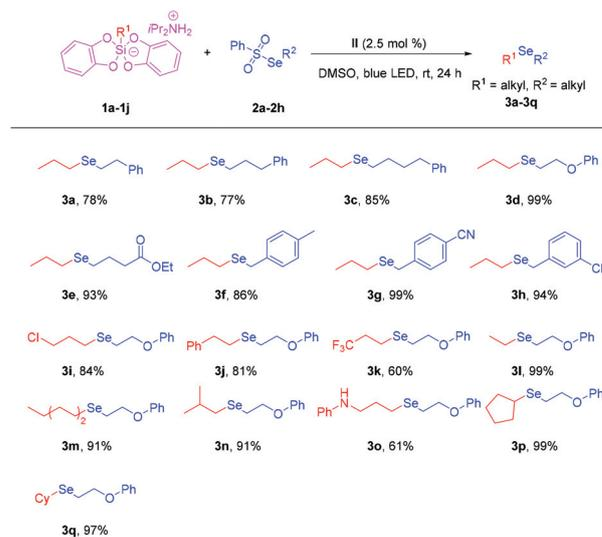
**Scheme 2** Substrate scope for unsymmetrical alkyl-alkyl selenide compounds. Reaction conditions: substituted silicate **1** (0.34 mmol), substituted selenosulfonates **2** (0.2 mmol), **II** (2.5 mol%), (dry) DMSO (1 mL), room temperature, blue LED, N<sub>2</sub>, 24 h. Isolated yields.
