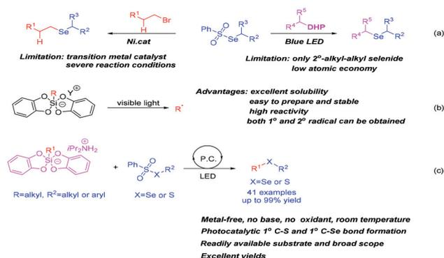
**Scheme 1** (a) Ni-catalyzed C–Se bond construction and C–Se bond construction under photocatalysis. (b) Hypervalent silicon compounds as a source of C-radicals. (c) Visible-light-promoted free radical cross coupling of hypervalent bis-catecholato silicon compounds with selenosulfonates or thiosulfonates.
